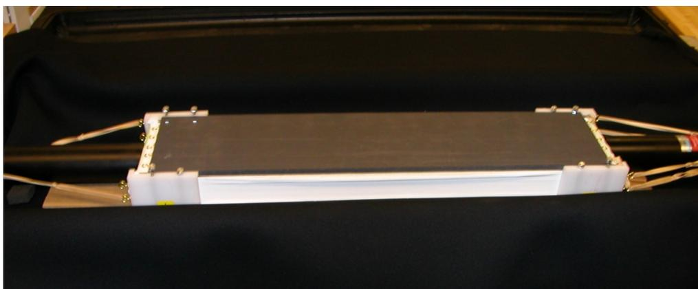
**Figure 7. Bench-top test unit assembled on a support structure with two PMTs and no tapered light guides.**
