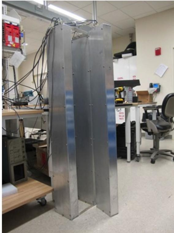
**Figure 32. Demonstrator system of four paddles (three are visible) ready for insertion of the source for measurements.**
