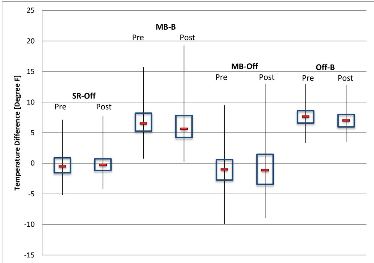
**Figure 3.2.** Average temperature difference between the sunroom and office (SR-Off), master bedroom and basement (MB-B), master bedroom and office (MB-Off), and office and basement (Off-B) during the baseline (pre) and post-fenestration retrofit (post) periods. The maximum and minimum temperature differences are represented by the solid black lines (whiskers) and the blue boxes mark the upper and lower quartile of the temperature differences.
