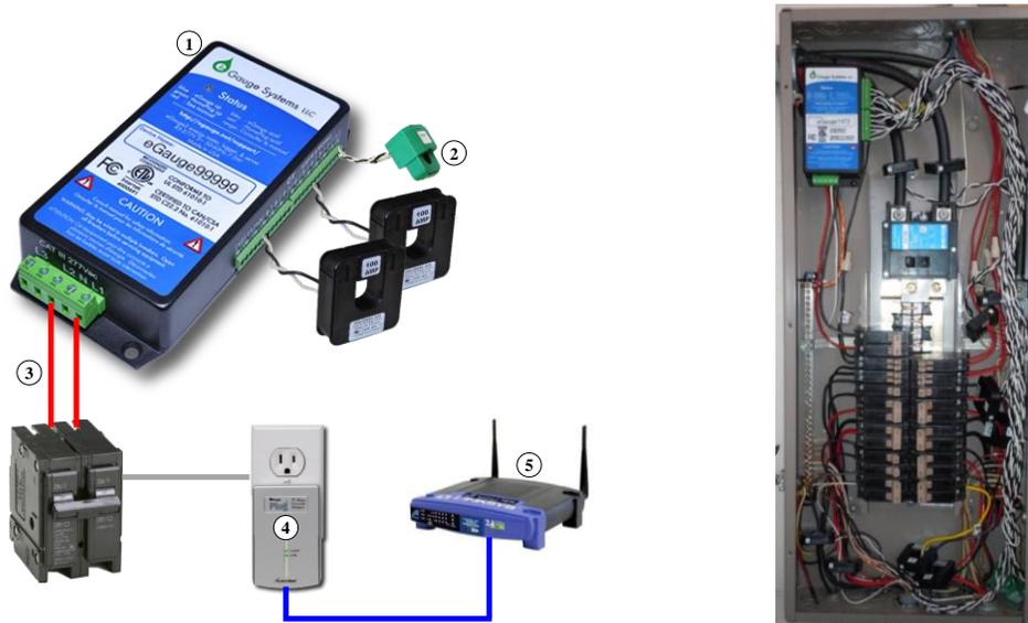
**Figure 2.3.** Schematic and photograph of an eGauge energy metering system, consisting of a 1) main power meter unit, 2) current transformers, 3) voltage taps connected to a dual-pole breaker, 4) HomePlug communication adapter, and 5) an Internet router. Note that the HomePlug and Internet router are not shown in breaker panel photograph.
