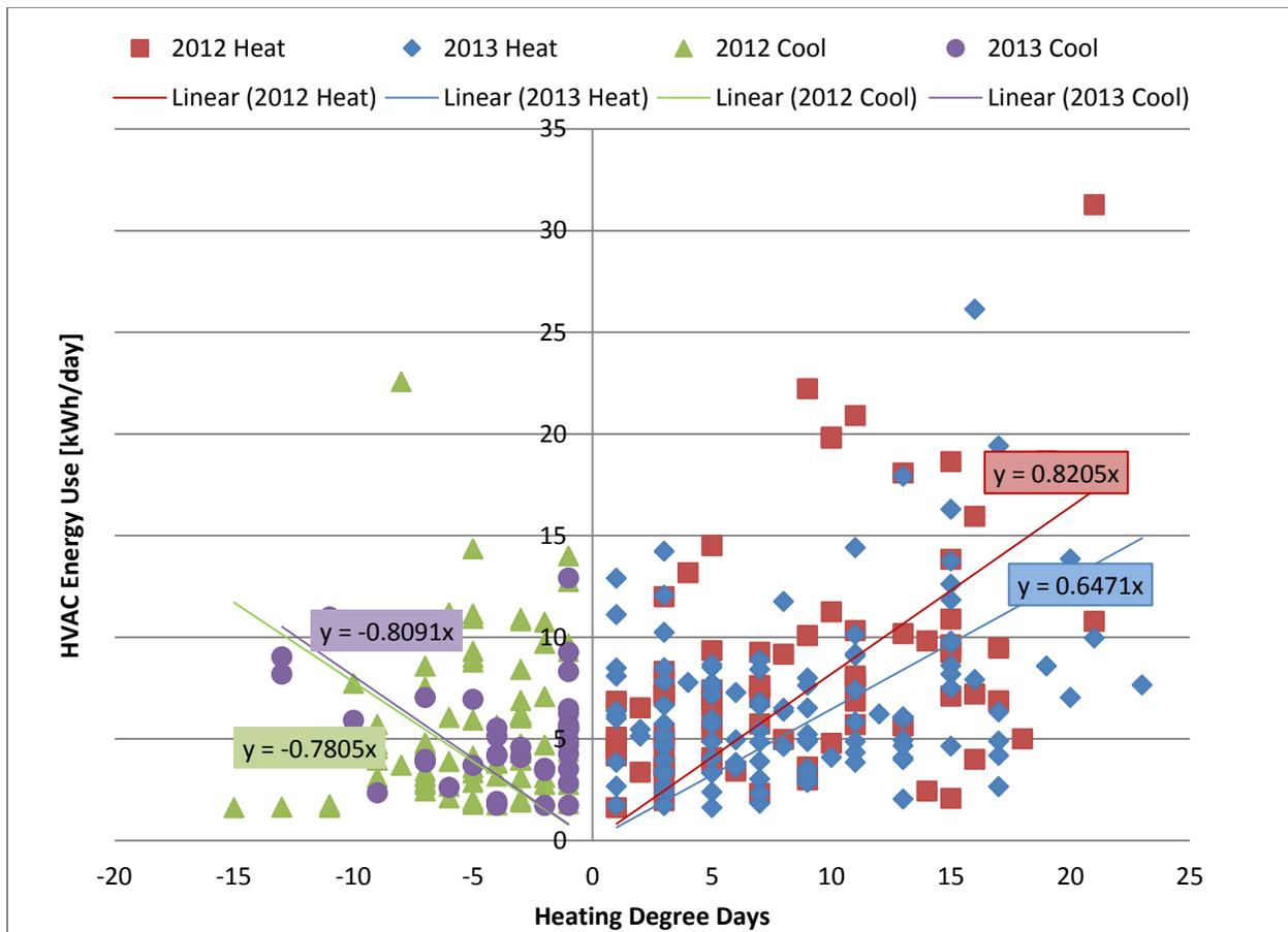
**Figure 3.1.** Daily HVAC energy use from April 1st through September 17th for the baseline period (2012; red and green) and post-fenestration retrofit (2013; blue and purple) normalized based on measured HDDs/CDDs for that period, where HDDs are positive numbers and CDDs are negative numbers.
