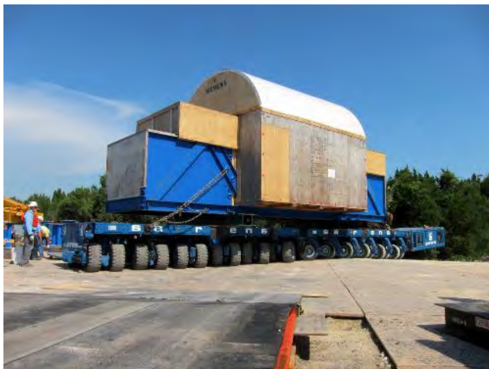
Figure 2-198. Self-Propelled Modular Transporter Turning with Turbine Components (2012)
