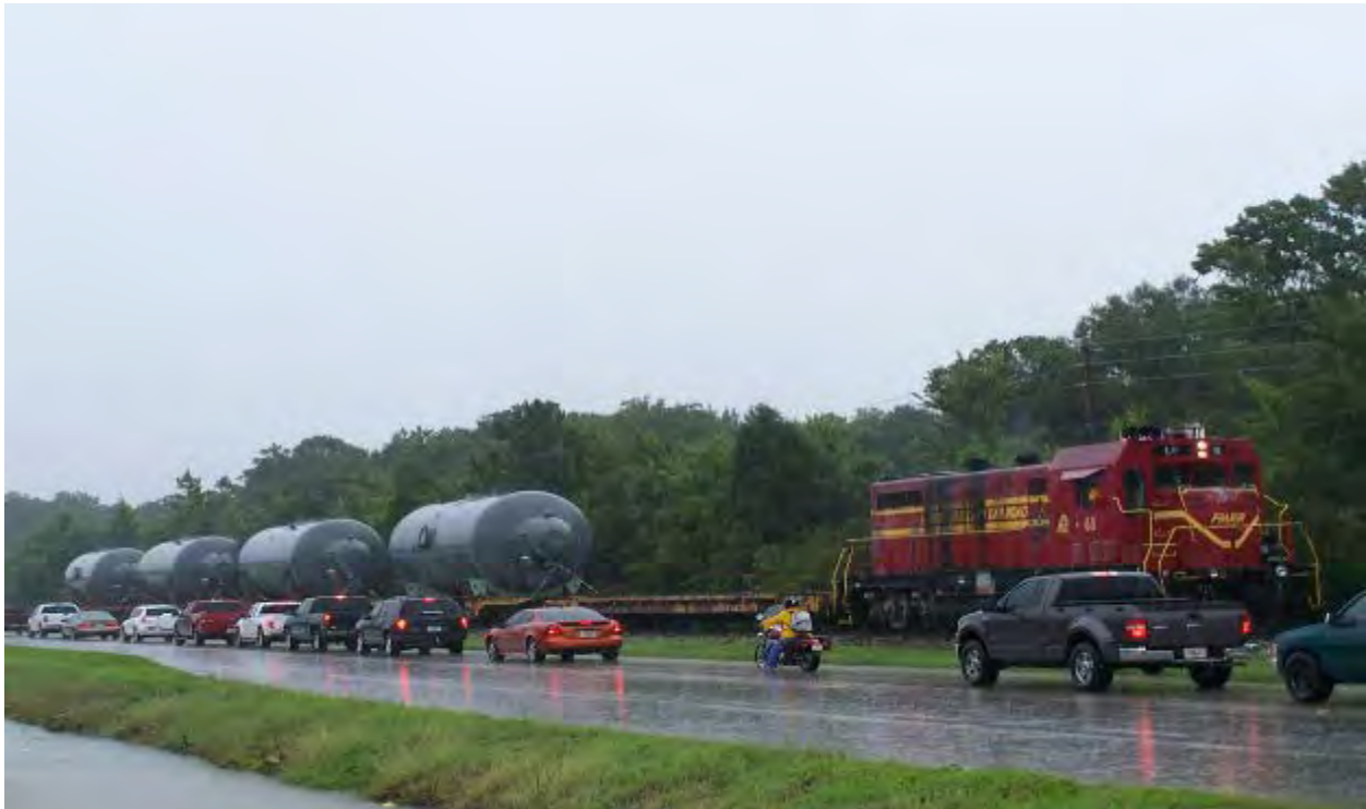
Figure 2-180. Moisture Separator Reheaters Being Shipped by Rail to the Crystal River Site (2009)
