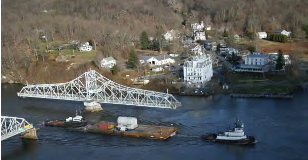
Figure 2-45. Connecticut Yankee Reactor Pressure Vessel Being Transported on Barge in the Connecticut River
