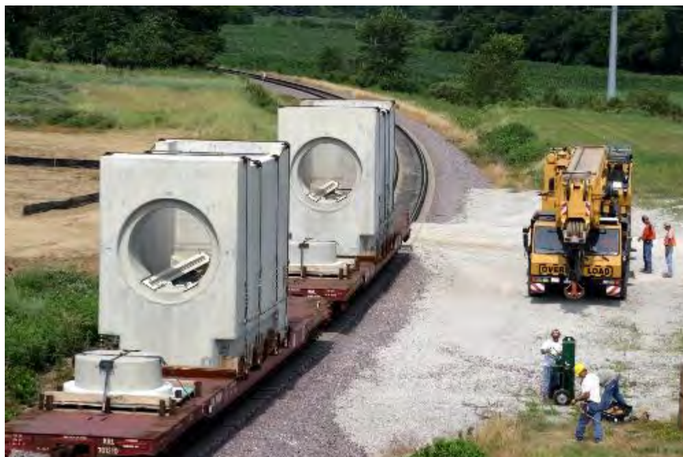
Figure 2-355. Horizontal Storage Modules Being Delivered to Fort Calhoun
