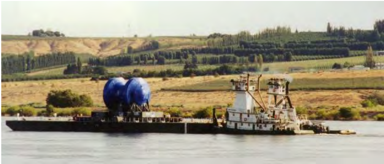
Figure 2-116. Trojan Reactor Pressure Vessel Being Transported by Barge (1999)
