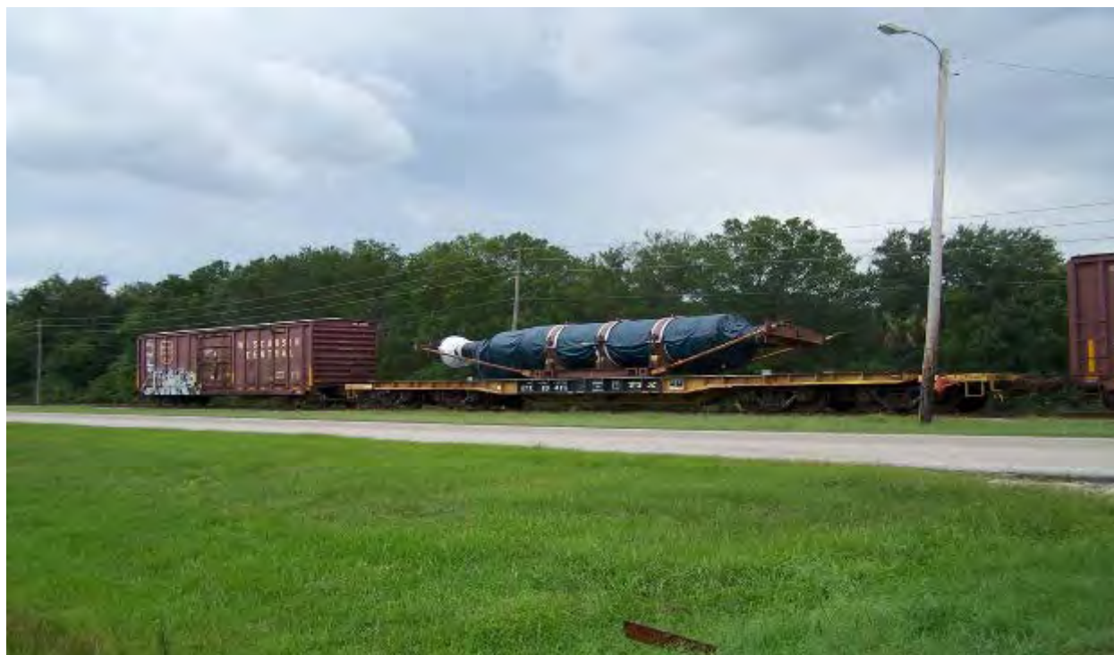
Figure 2-182. Generator Rotor Being Shipped by Rail to the Crystal River Site (2009)
