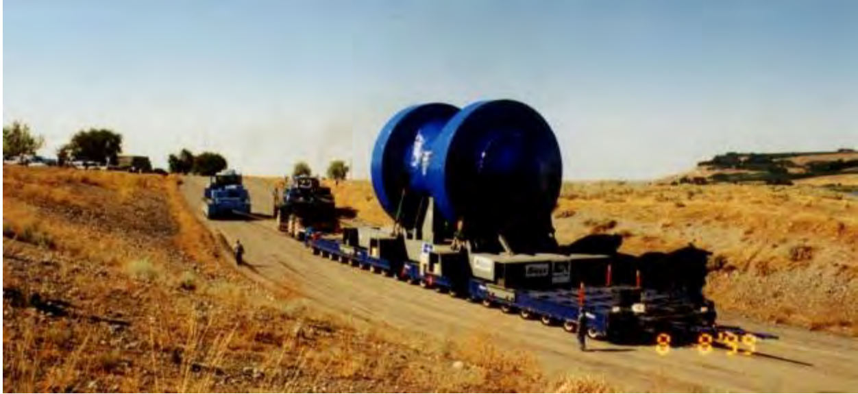
Figure 2-118. Trojan Reactor Pressure Vessel Being Transported by Heavy Haul Truck (1999)
