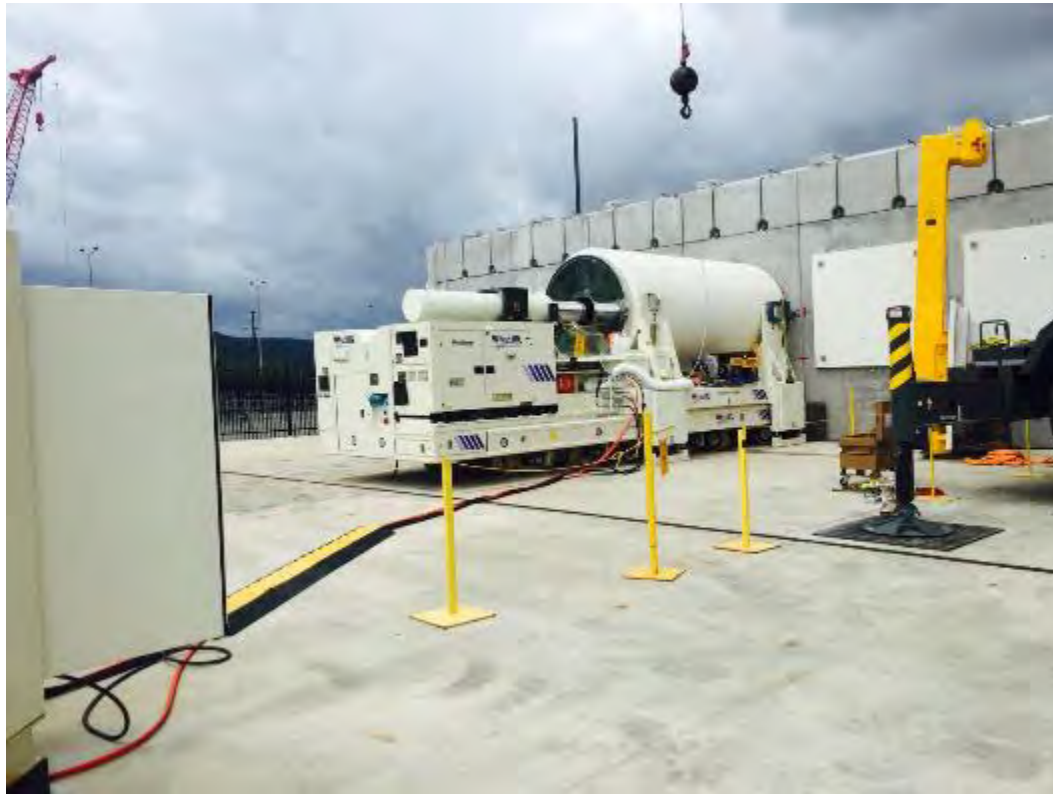
Figure 2-152. Transfer Cask Being Used to Load Canister into Horizontal Storage Module
