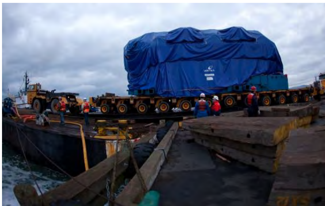
Figure 2-54. Wartsila Engine Being Loaded on a Barge (2010)
