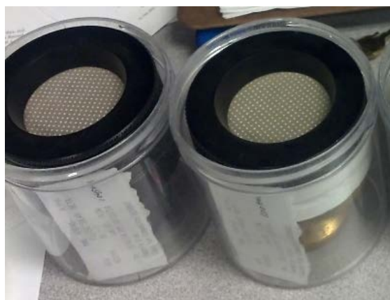
Figure 8. Example of Two Exposed Air Particulate Filter-Head Assemblies Prior to Analyses
