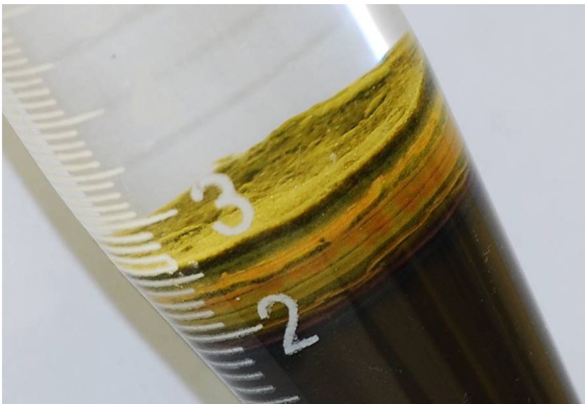
Figure 3.7. Test 6 Side/Upper View on 14 July 2010 After 287 Days of Oxygenated Water Exposure. Sample tilted to the left about 35° from vertical.
