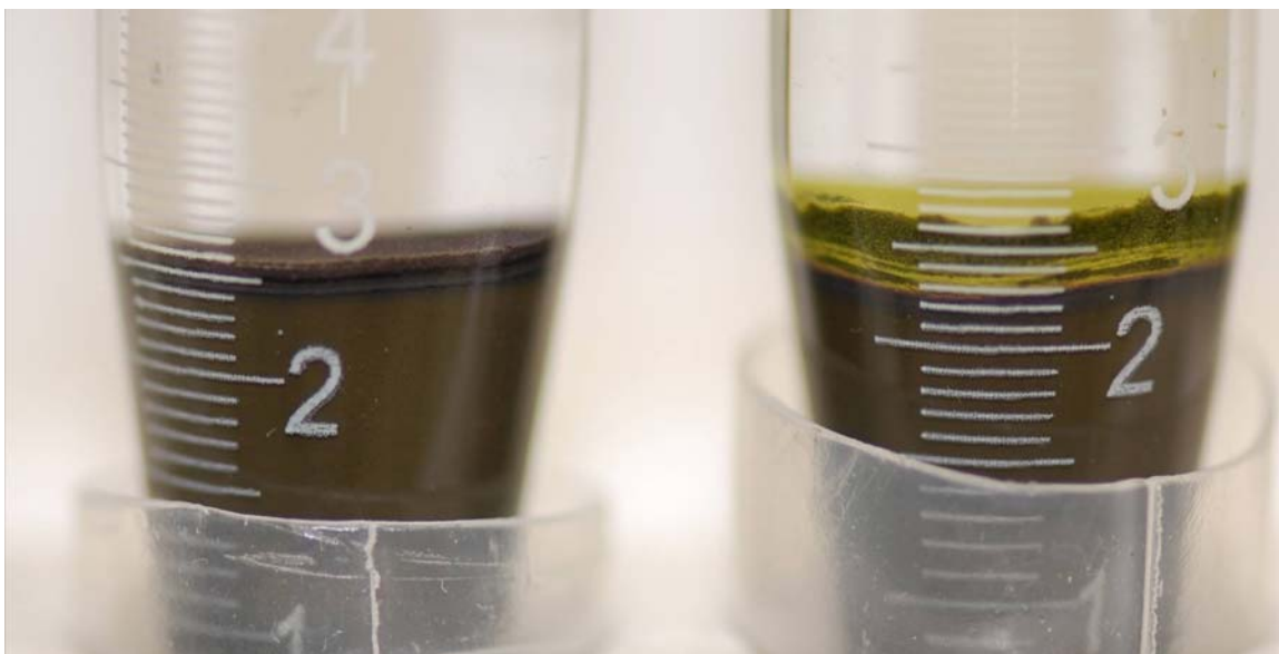
Figure 3.3. Appearance on 1 December 2009 after 62 Days Left: Control starting \text{UO}_2 settled slurry, not exposed to oxygenated water Right: Test 2 \text{UO}_2 slurry after 71 days of oxygenated water exposure
