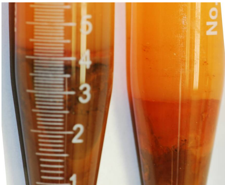
Figure 3.20. S-Control and S-4 Tests after 106 Days of Exposure to 51°C Oxygenated Water
