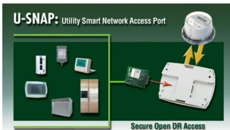
Figure 3. The U-SNAP Vision to Enable Communication between HAN Devices and an AMI Smart Meter is Agnostic of the Underlying Communication or Messaging Protocol (U-SNAP 2009b)
