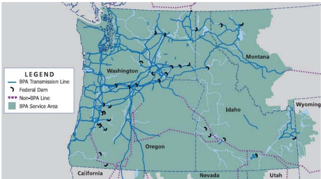
Figure 1. The BPA Service Area with Transmission Lines and Federal Dams<sup>1</sup>
