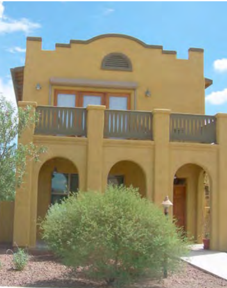
Building America partner John Wesley Miller's homes at Armory Park del Sol beat the Building America benchmark by 50% thanks in part to a building envelope that includes masonry walls with external rigid insulation and R-38 attic insulation.
