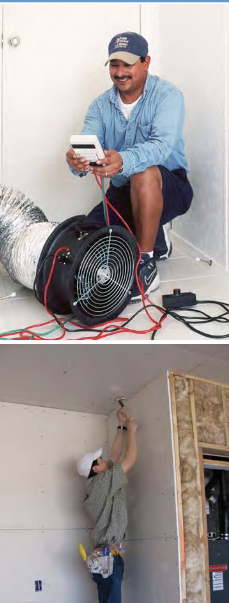
(top) Duct blaster testing confirms that ducts are well sealed (Source: NREL)
