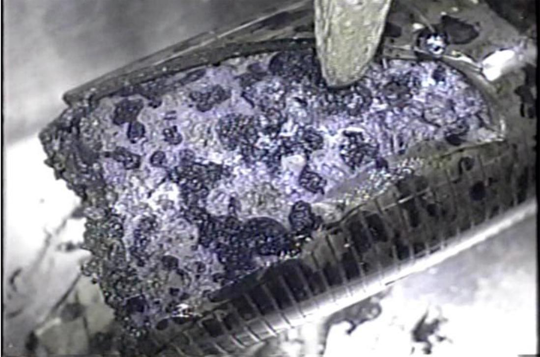
**Figure 4.3.** Sample 96-13 Shear Strength Estimate 2. Start of forceps impingement.
