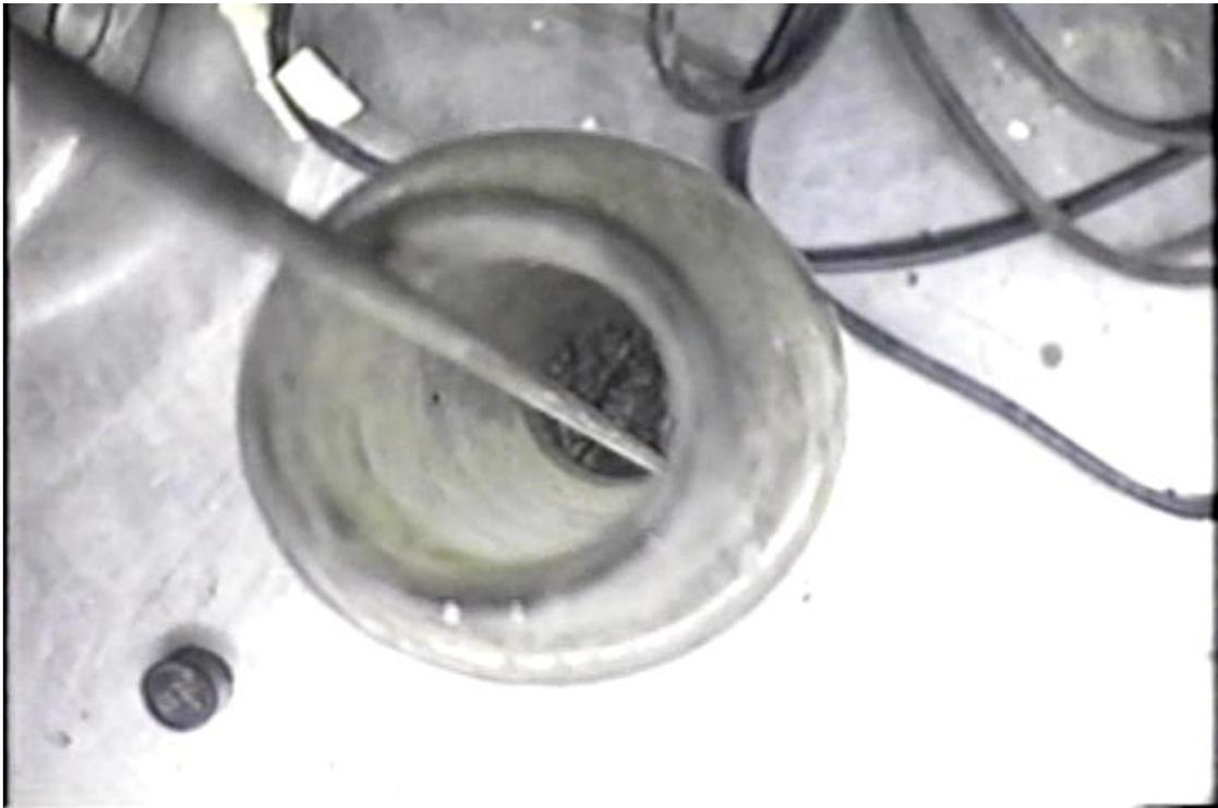
**Figure 4.2.** Sample 96-13 Shear Strength Estimate 1. Spoon blade is at lower right; “imprint” of spoon blade tip appears to be visible at center.
