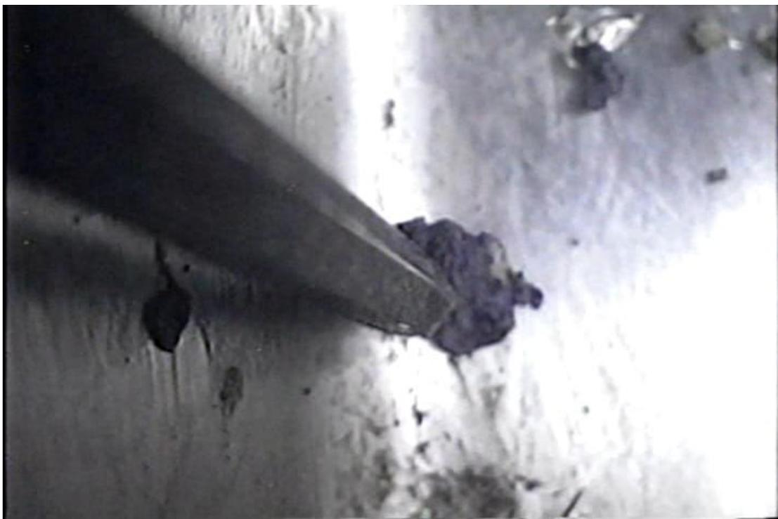
**Figure 4.10.** Sample 96-13 Shear Strength Estimate 5. Hex wrench placement.
