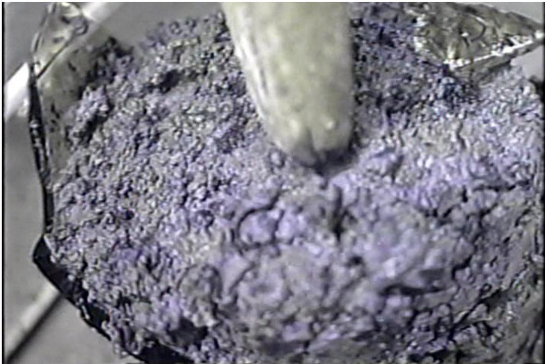
**Figure 4.5.** Sample 96-13 Shear Strength Estimate 3. Start of forceps impingement.
