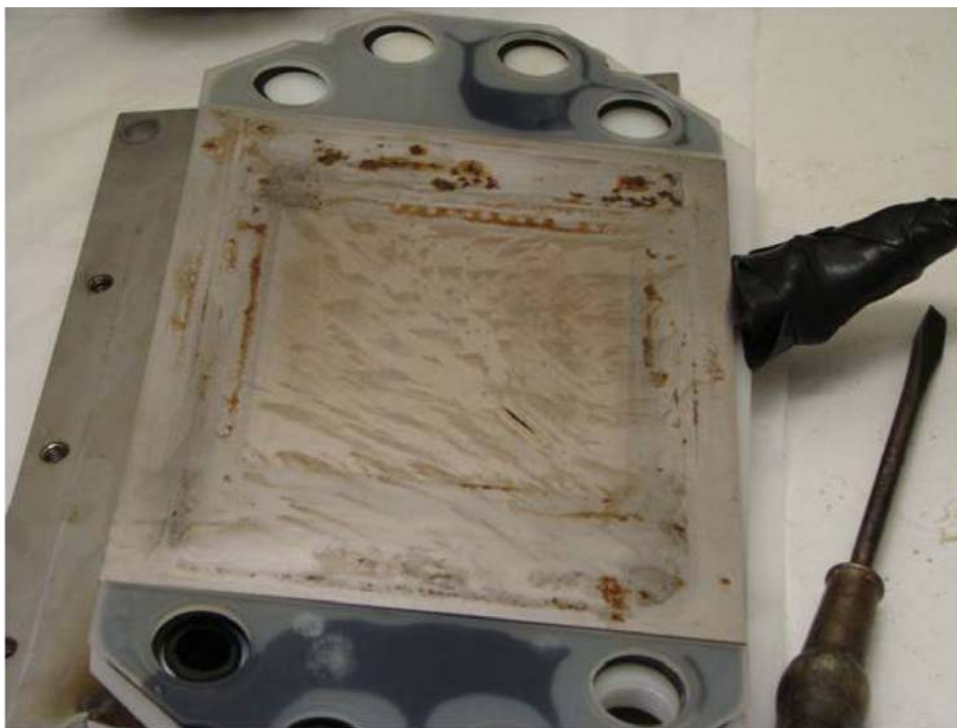
Figure A.5. Membrane Side of the Kovar ™ Electrode. Discoloration Appears to Be Corrosion Byproducts
