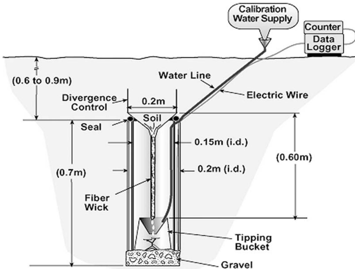
**Figure 2.1** Schematic of installed vadose zone water fluxmeter with diversion control (Gee et al. 2002)
