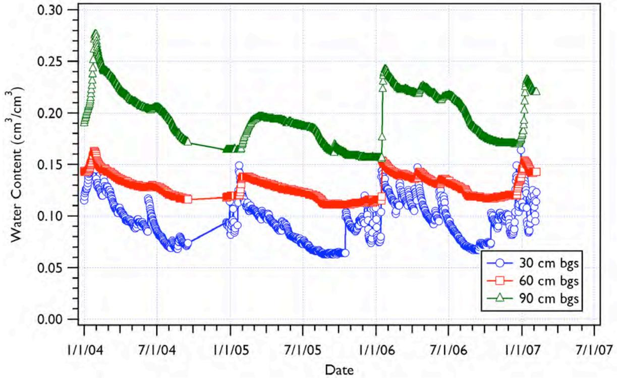
**Figure 4.51** SX Pit Measured Water Content at 30, 60, and 90 cm bgs
