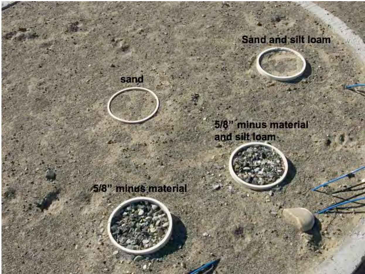
**Figure 4.48** Photograph of One of the Four Cement Caissons at the FLTF Pit Showing WFMs Packed with Different Materials
