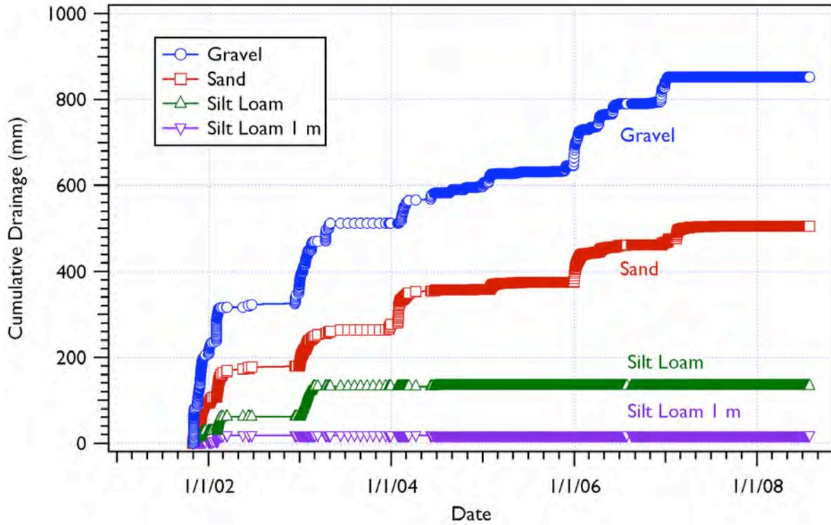
Figure 4.49 FLTF Pit WFM Measured Drainage for Sand, Silt Loam, and Gravel Treatments
