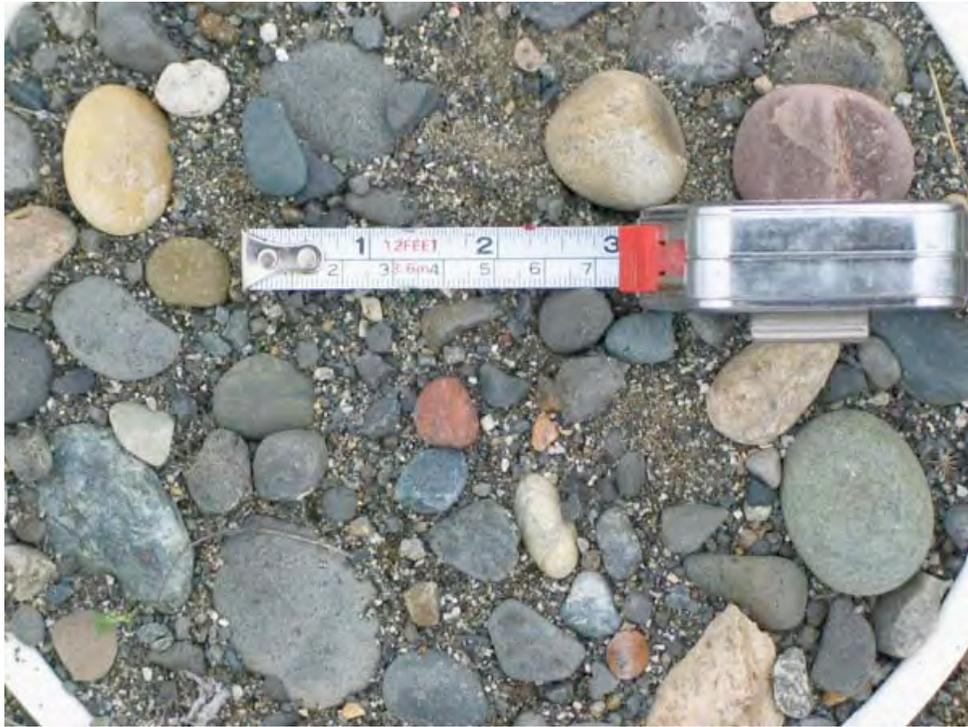
**Figure 4.15** WFM Material at the Hanford SWL
