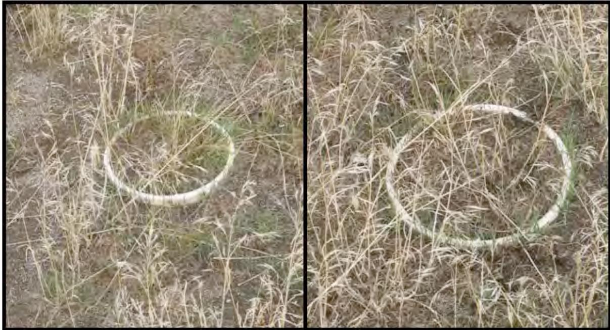
**Figure 4.2** Surface Conditions of the Grass Site WFMs in Autumn 2006 (exposed tops of these WFMs are the identically sized at 20-cm diameter, but appear different sizes because of camera distance)
