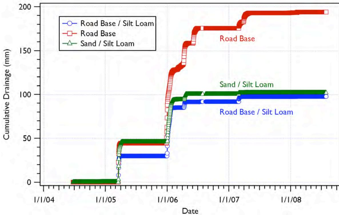
Figure 4.50 FLTF Pit WFM Measured Drainage for Road Base/Silt Loam, Road Base, and Sand/Silt Loam Treatments
