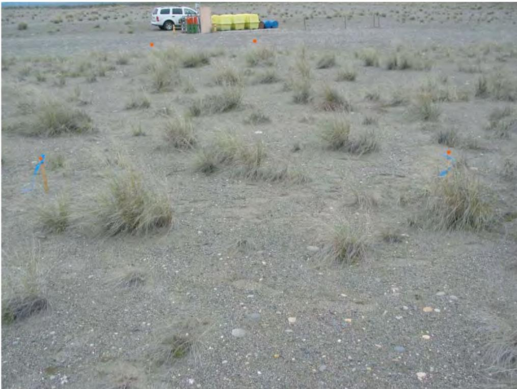
**Figure 4.16** SWL Basin Lysimeter (orange dots represent approximate corners of the basin lysimeter)
