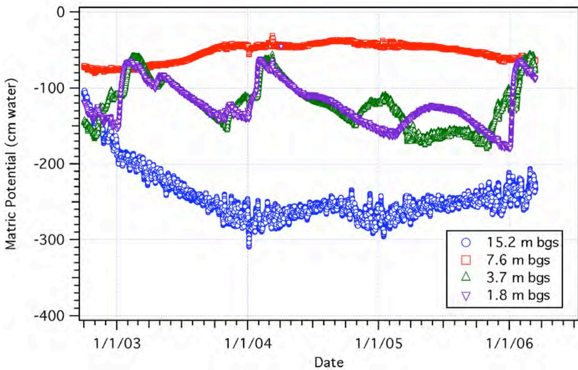
**Figure 4.54** TX Tank Farm Matric Potentials at Four Depths Since Installation
