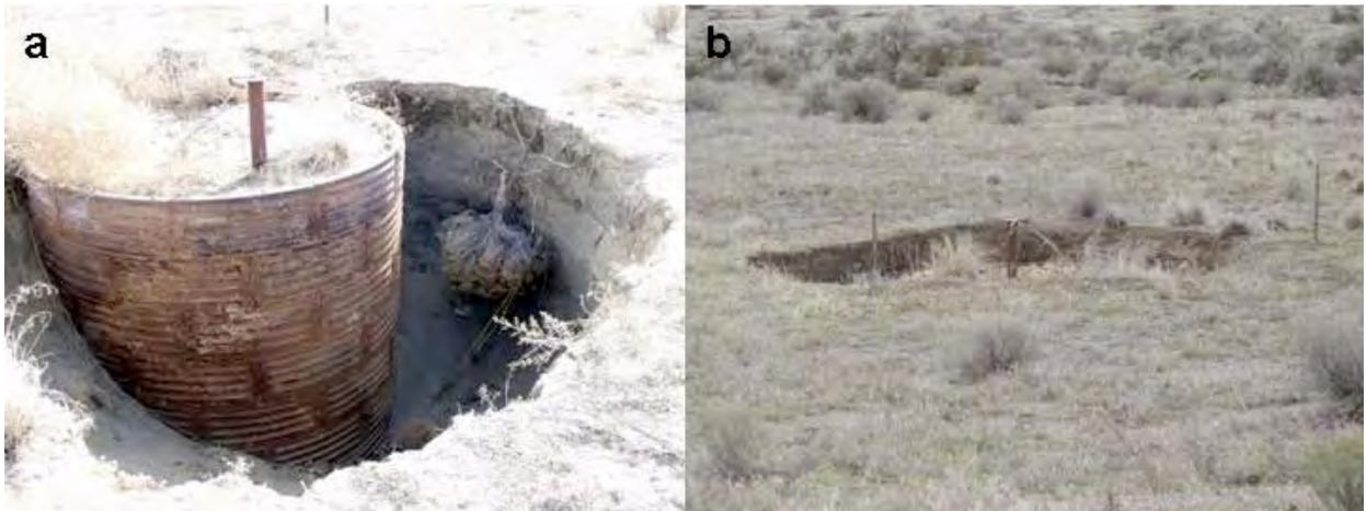
**Figure 4.28** 200 East Lysimeter Subsidence; Image b Shows the Subsidence From a Distance (photograph taken after discovery of soil subsidence in 2005)
