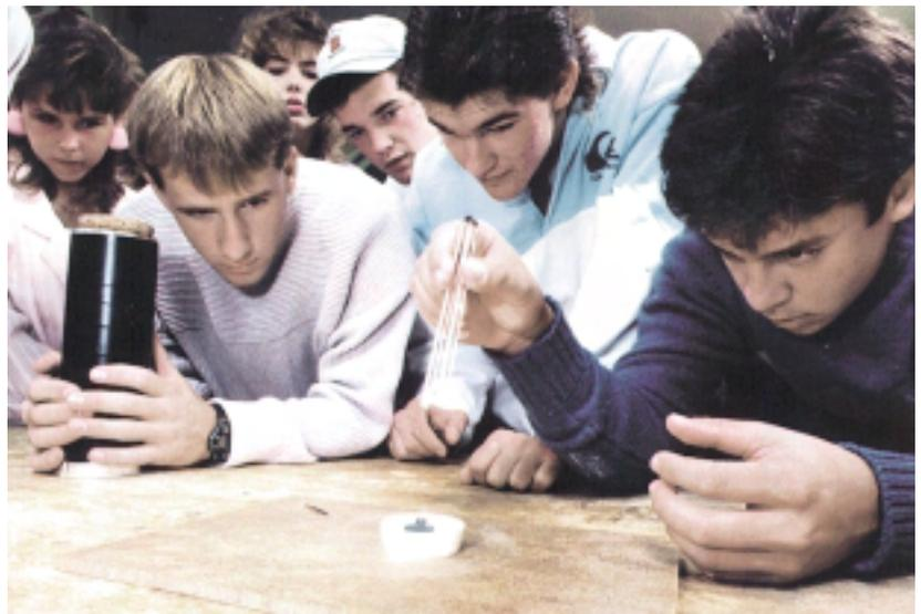
1. Attach the micro-ohmmeter (four-point type) to a pellet and take a resistance reading at room temperature. Now submerge the pellet in liquid nitrogen, and take a second reading. In its cooled state, the resistance measurement should read zero ohms. (Readings from this measurement can be erratic due to poor contact or high-contact resistance).
