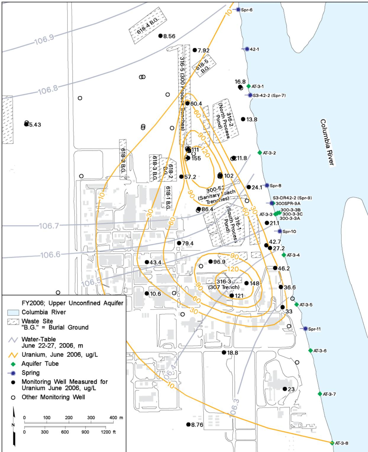
**Figure 2.13.** Water-Table Elevations and Uranium Concentrations in Upper Part of Unconfined Aquifer Beneath the 300 Area, June 2006 (Source: Hartman et al. 2007)
