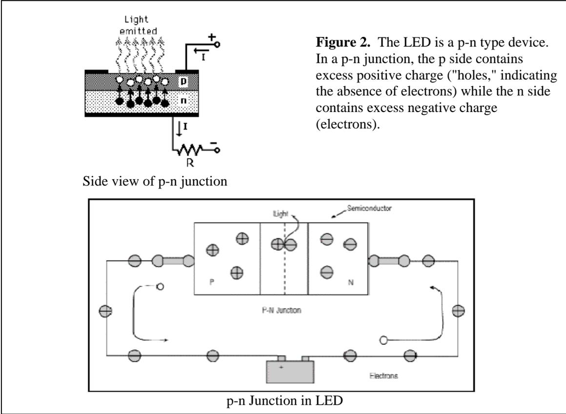
**Figure 2.** The LED is a p-n type device. In a p-n junction, the p side contains excess positive charge ("holes," indicating the absence of electrons) while the n side contains excess negative charge (electrons).
