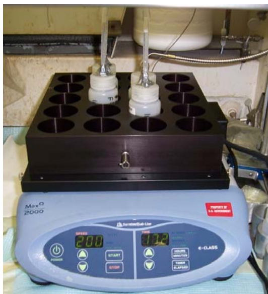
Figure 7.1. Batch Contact Shaker Supporting Parametric Testing
