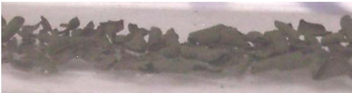
Figure D.1. Digital Picture of the Caustic-Leached, Water-Washed G6-Cr-TGA Sample Before TG Experiments
