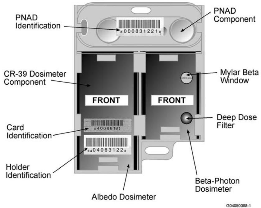
**Figure 5.16** Hanford Combination Neutron Dosimeter with PNAD
