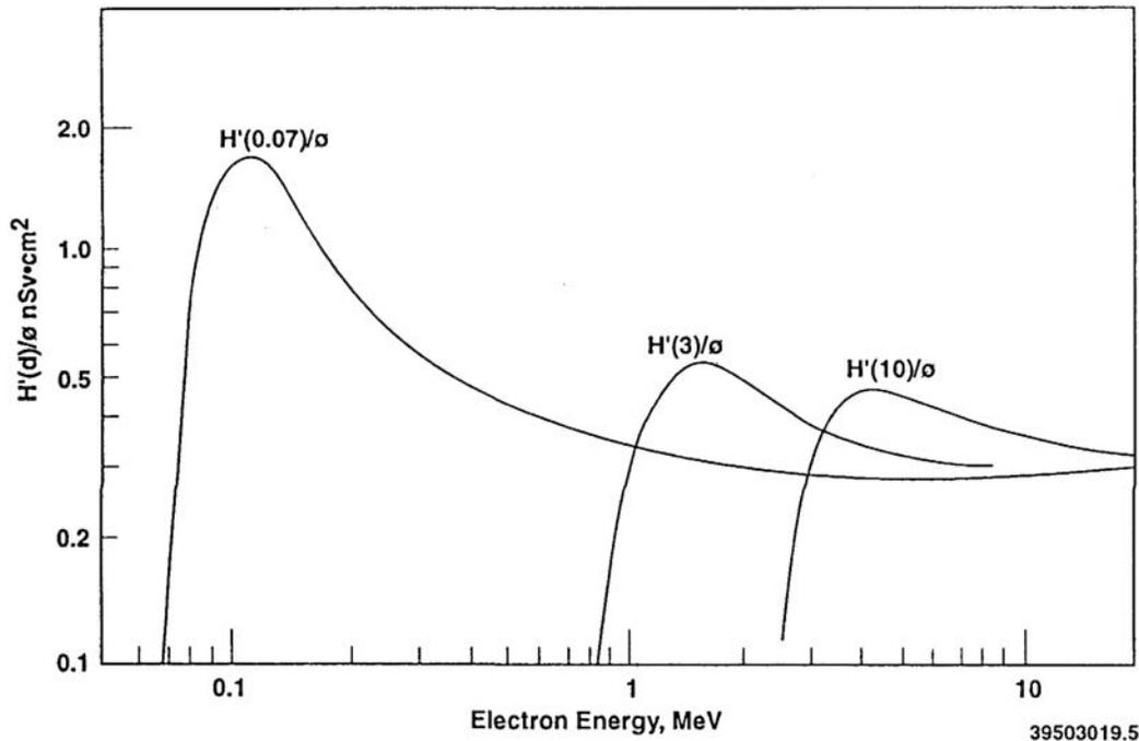
**Figure 6.1.** Variation in Dose Equivalent for Beta Radiation
