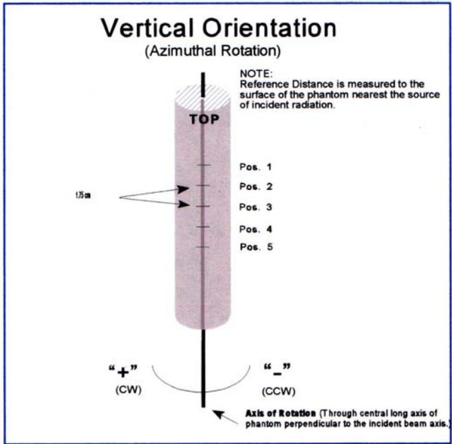
**Figure 5.29** Ring Orientation for Angular Dependence Irradiations
