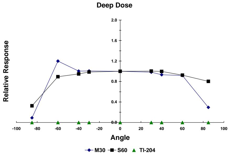
**Figure 5.11.** HSD Angular Response – Horizontal Rotation
