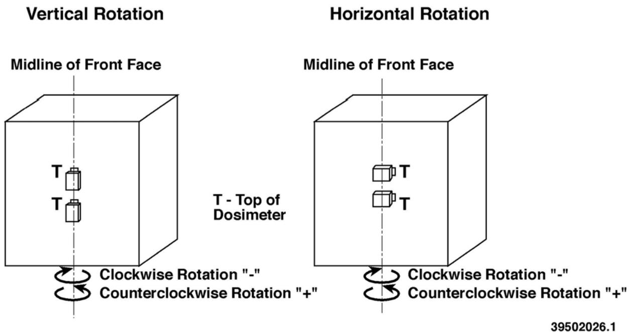
**Figure 5.8.** Irradiation Setup for Dosimeter Angular Response Evaluation
