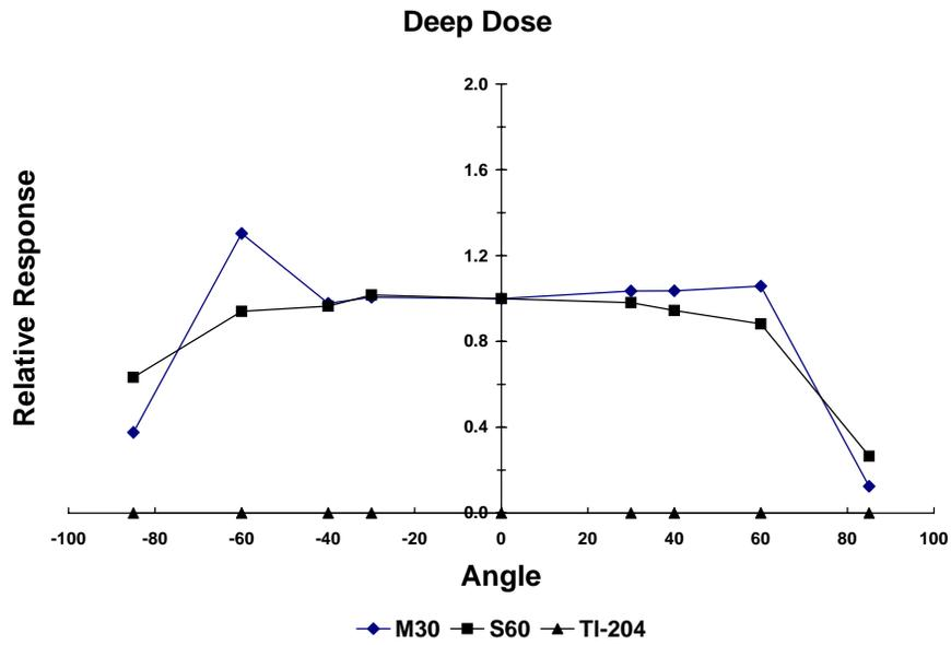
**Figure 5.12.** HSD Angular Response – Vertical Rotation
