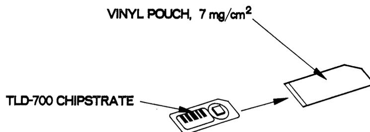
**Figure 5.36** Illustration of Chipstrate Sealed in Vinyl Pouch
