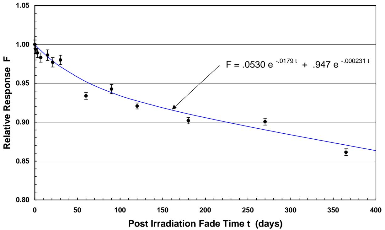
**Figure 5.26** Fade Correction for the Hanford Ring
