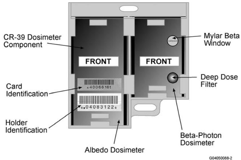
**Figure 5.17** Hanford Combination Neutron Dosimeter without PNAD
