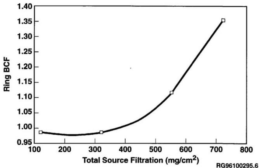
Figure 5.31 Ring BCF vs. <sup>90</sup>Sr/<sup>90</sup>Y Source Filtration
