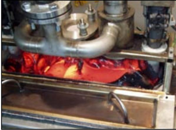
*At the Radiochemical Processing Laboratory, this setup was used to conduct engineering-scale bulk vitrification tests on technetium-99 spiked simulants.*
