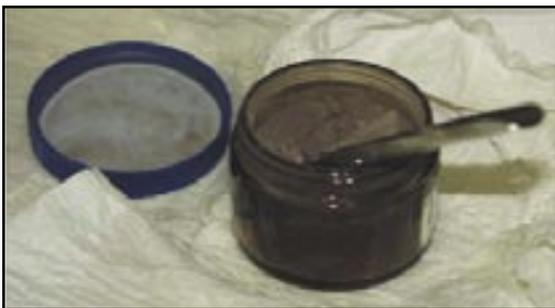
*During FY04, PNNL completed its analysis of unleached sludge from tank BX-101. Several of the tests showed that some tank waste contaminants were not as leachable as previously thought.*
