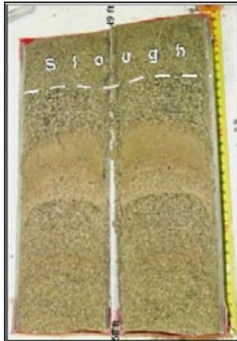
*Geochemical analysis of cores collected from the 200 Area of the Hanford Site has highlighted the effect lenses of fine-grained material have on the mobility of subsurface contaminants. Differences in the hydraulic conductivity of the fine-grained material and the overlying sand can lead to the horizontal migration of contaminants hundreds of meters from the tanks.*
