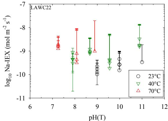
**Figure 12.** Na-IEX Rate as a Function of Solution pH and Temperature
