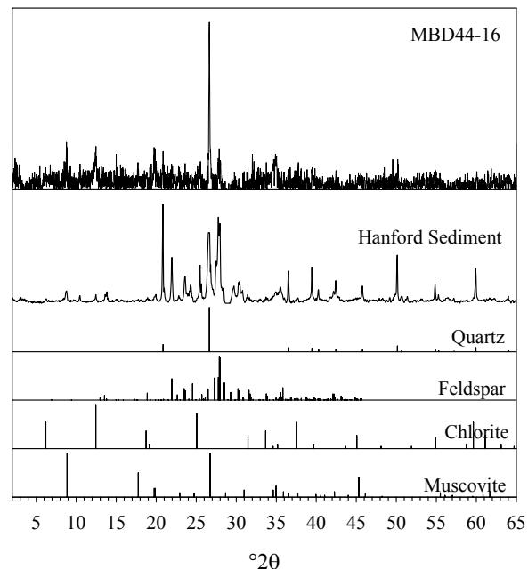
**Figure 37.** Comparison of XRD Patterns for Reacted Solids Removed After 700 days from Test MBD44-16 and Hanford Soil
