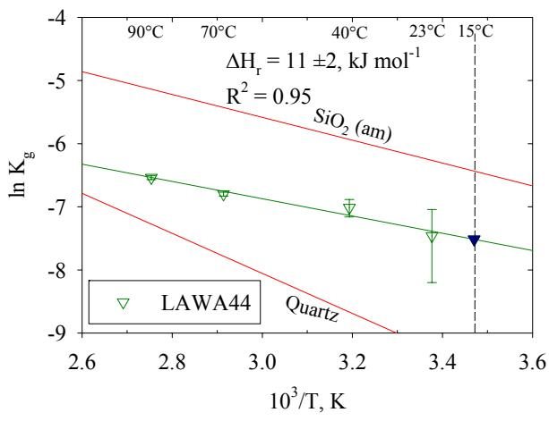
**Figure 7.**  $\ln K_g$  vs. Inverse Temperature for LAWA44 Glass
