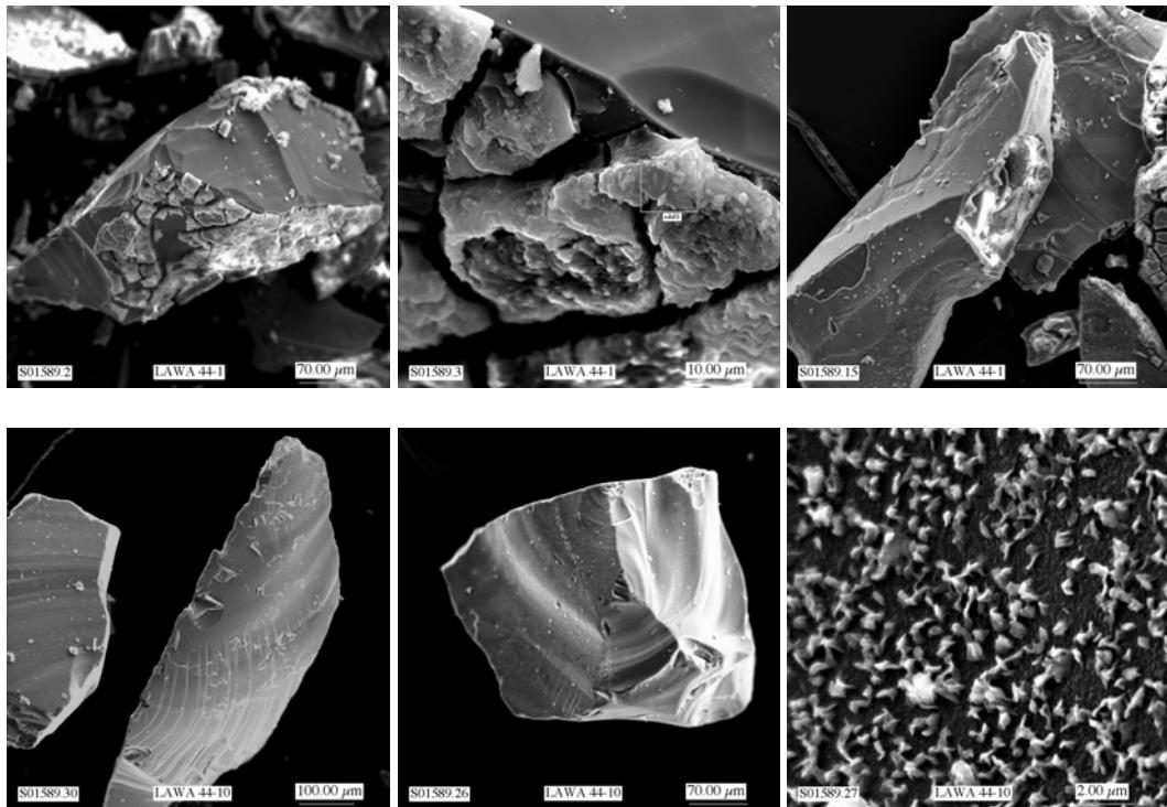
**Figure 21.** SEM Photographs of Reacted Grains of LAWA44 Glass After 858 Days in PUF Test at 2  $\text{mL}/\text{d}$  and 99°C. The first row of pictures is from sample S1 at the column inlet. The second row is from sample S10, 44 mm downstream from the column inlet.
