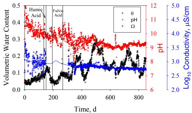
**Figure 18.** Computer Monitored Test Metrics From PUF Tests with LAWA44 Glass. Lines are bi-square smoothed fits to the raw data. The vertical lines give the periods where a  $50 \text{ mg/L}$  humic acid solution and a  $10 \text{ mg/L}$  fulvic acid solution was injected instead of deionized water.
