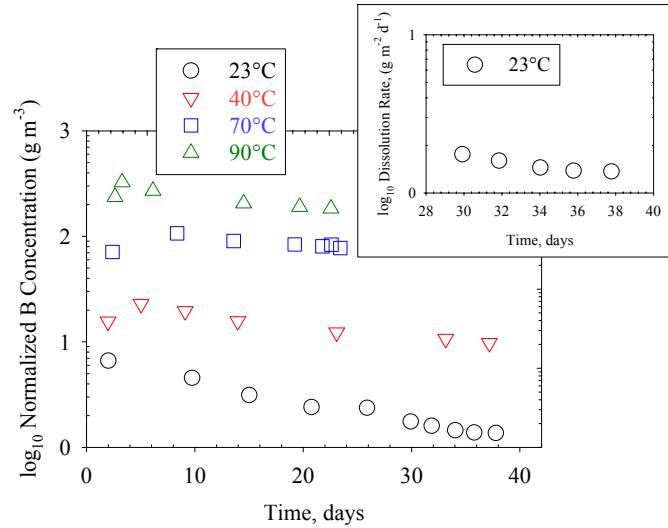
**Figure 2.** Normalized B Concentration as a Function of Time and Temperature for LAWA44 Glass with Increased Resolution for the  $23^\circ$ C Results Between Day 30 and 38.
