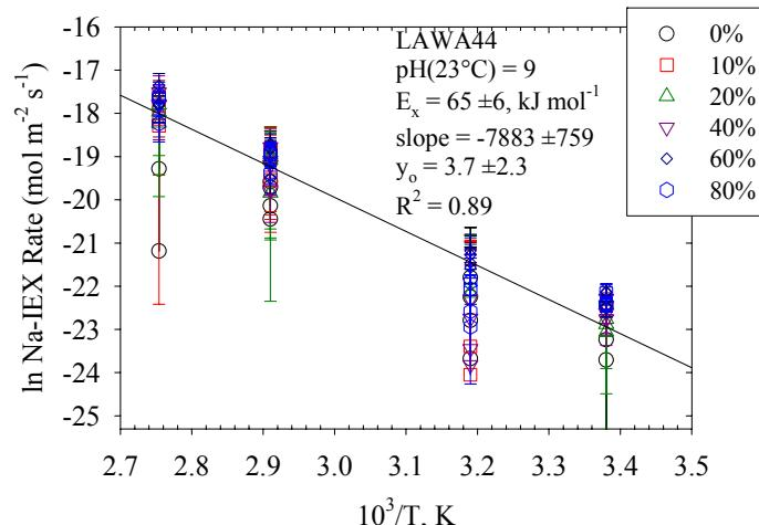
**Figure 5.** Na Ion Exchange Rate as a Function of Temperature with Changing a[SiO<sub>2</sub>(aq)] for LAWA44 Glass
