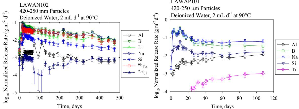
**Figure 28.** Normalized Release Rate for Selected Elements in PUF Test with LAWAN102 (left) and LAWAP101 (right) Glasses.
