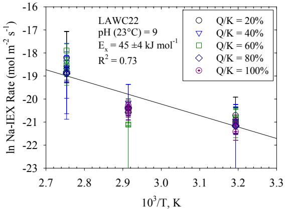
**Figure 13.** Na Ion Exchange Rate as a Function of Temperature with changing  $a[\text{SiO}_2(\text{aq})]$  for LAWC22 Glass
