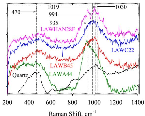
**Figure 17.** Raman Spectra of LAWA44, LAWB45, LAWC22 and Reference spectra for Quartz
