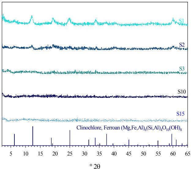
**Figure 22.** XRD Analyses of Reacted LAWA44 Glass Samples Taken from PUF Column After 859 days at  $2\text{ mL d}^{-1}$  and  $99^\circ\text{C}$ .
