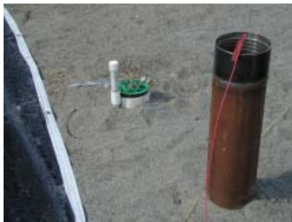
Photo 2 – SW Steel casing and ERT sensor
