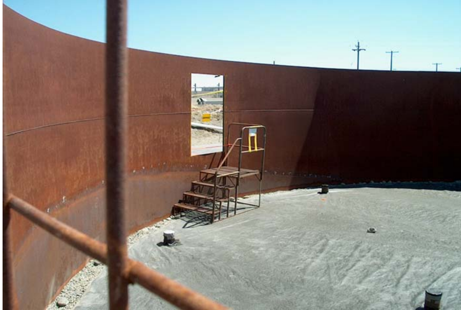
Figure 7. Interior Access to the Mock Tank. A door was cut in the east side of the tank and stairs installed to the floor of the tank (~0.9 m [~3 ft] below exterior grade). This allowed installation of instruments and monitoring of soil conditions beneath the tank floor. The covering on the floor prevents air leakage during SAFE operations. Three of the 12 soil access ports are shown protruding from the floor covering.
