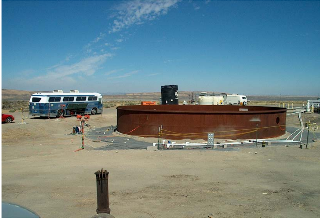
Figure 5. View Looking East at the Mock Tank During the FY 2001 TLDD Activities. Large PVC pipes are SAFE air-extraction lines. The bus at left is the mobile geophysics laboratory. The large black storage tank contains the sodium thiosulfate solution used to simulate a tank leak (see Section 2.4.4). The trailer and the RV to the right of the storage tank are the SAFE field laboratory.
