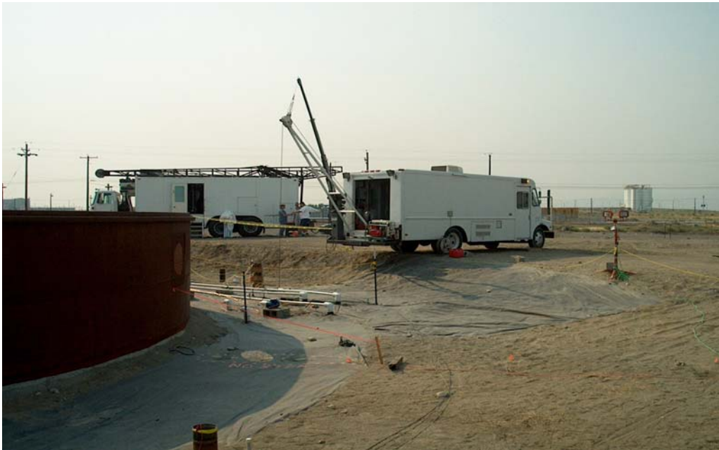
Figure 19. Receiving Coil for the CEMI Method Being Lowered into a Well. The transmitter is placed in a well opposite from the tank off the left side of the photograph. The truck housing the recording equipment and generator is seen in the background.
