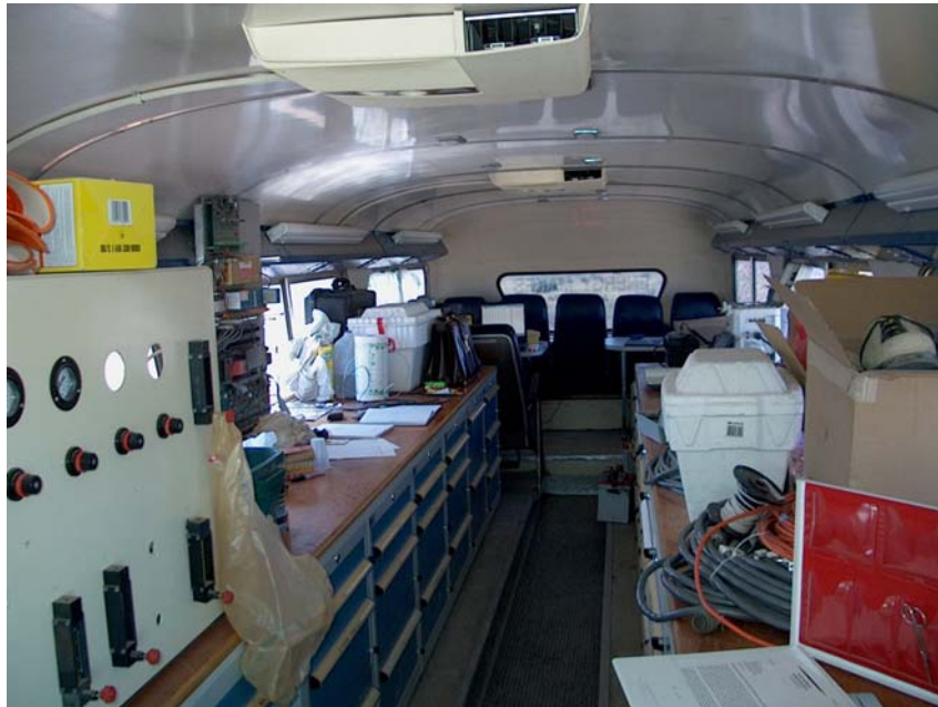
Figure 6. Interior of the Mobile Geophysics Laboratory Used for Workspace and Housing of Recording Equipment
