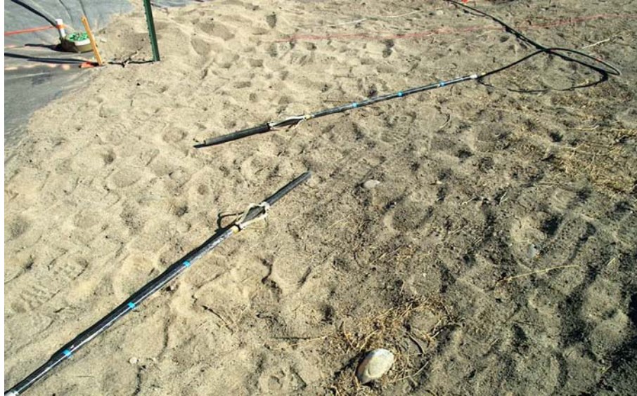
Figure 16. Antenna Configuration for XBR Measurements at the Mock Tank. Both transmitter and receiver are equipped with centralizers.
