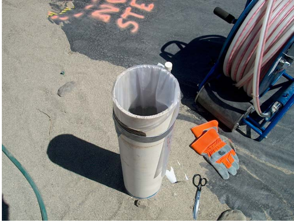
Figure 9. PVC Sealed Well Installed During FY 2001 with Liner Installed to Prevent Water Leakage. Seismic techniques require a water-filled well to provide sufficient coupling with the geologic formation and allow signal propagation.
