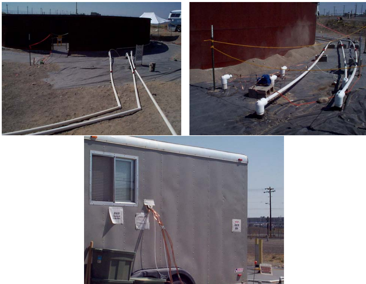
Figure 10. View of the SAFE Infrastructure Around the Mock Tank (top left and right), and Gas Monitoring and Sampling Lines Entering the SAFE Field Laboratory (bottom). Samples were analyzed by gas chromatography inside the laboratory. The SAFE experiments were conducted concurrently with the geophysical demonstrations.
