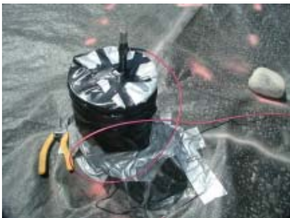
Photo 1 – Central injection electrode
