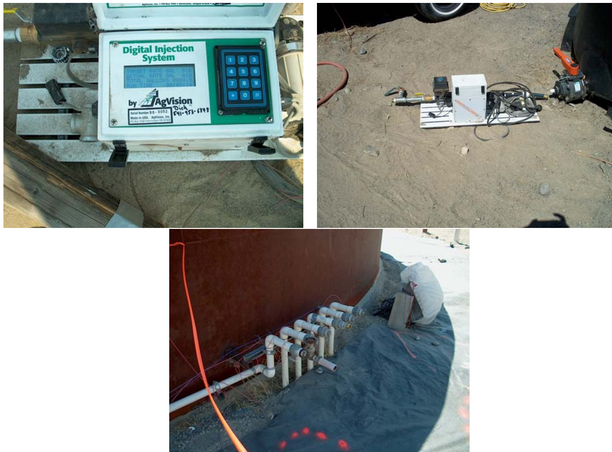
Figure 11. (Top and Middle) The Digital Flowmeter System Connected Directly to the 15,140-L (4000-gal) Sodium Thiosulfate Storage Tank; (Bottom) Existing Manifold System Used Initially to Deliver the Solution to the Central Leak Point in the Tank. This manifold was abandoned late in the test to circumvent suspected clogging.
