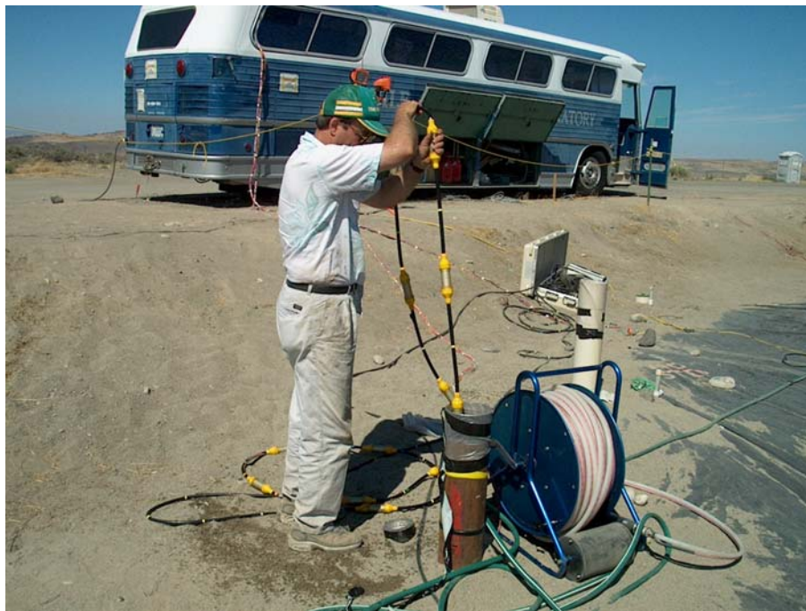
Figure 17. Lowering of Hydrophones (seismic receiver sensors) into a Steel Case-Lined Well at the Mock Tank. Wells were filled with water to perform the measurements, then pumped out after the measurements were finished (pump reel next to well)
