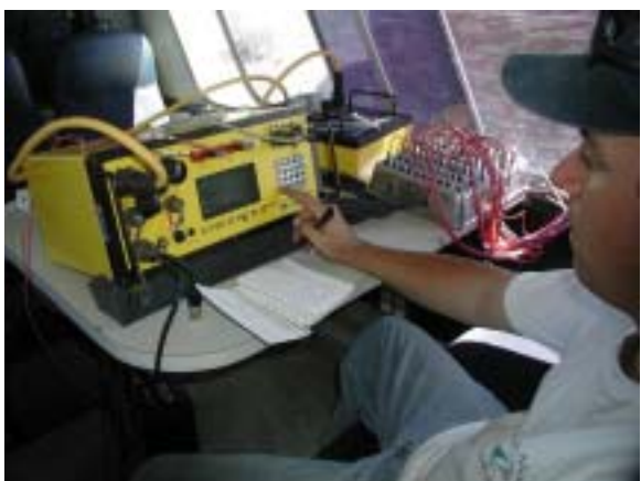
Photo 3 – AGI Sting R8, switch box, & patch panel
