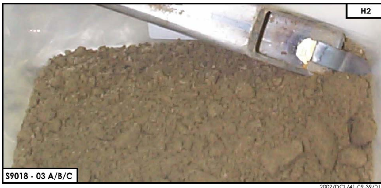
Figure 2.11. Lower Fine Sand and Mud Sequence of the Hanford Formation H2 Unit from Composite Sample S9018-03A, B, and C (at a depth of ~29 meters [95.5 feet]). Note tip of sidewall core sampler.
