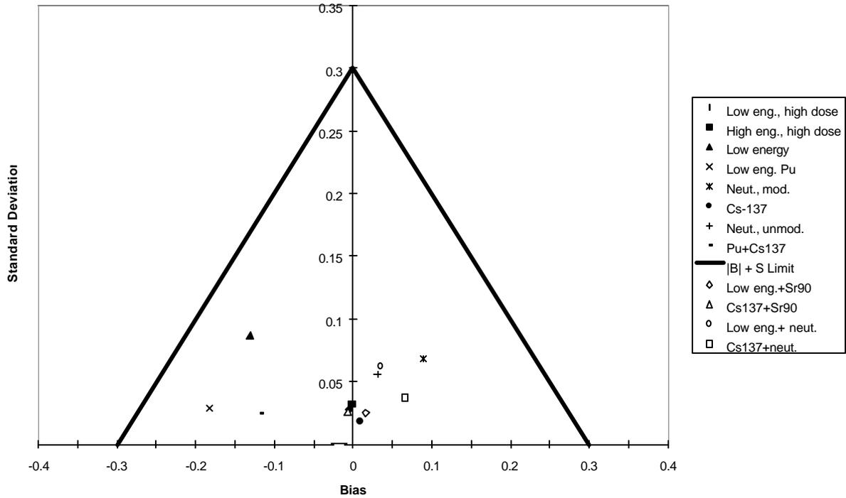
Figure 2.1. DOELAP Performance Results: HSD Whole Body Dosimeter, Deep Dose
