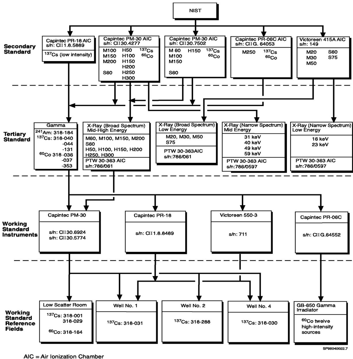
Figure 7.3. Typical Traceability Pathway for PNNL Photon Reference Fields
