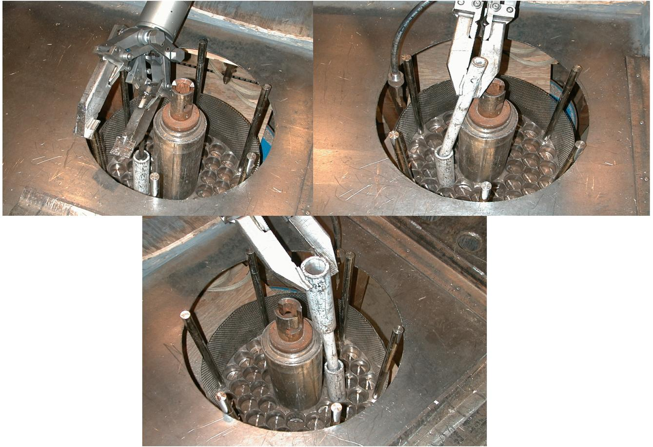
**Figure 10. Loading Broken Fuel Elements.**
