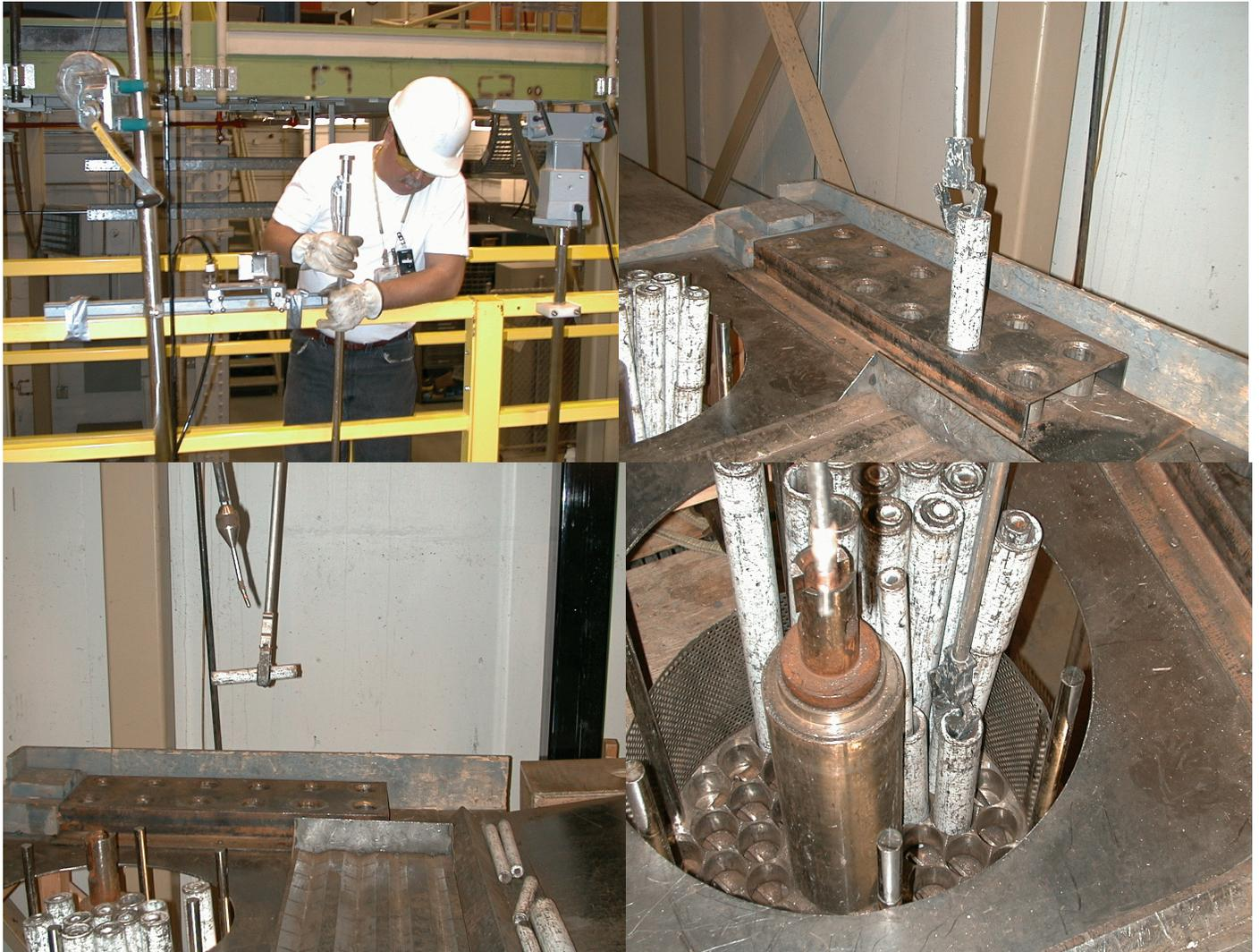
**Figure 8. Using the Modified Long Reach Gripper to Load Short Fuel.**
