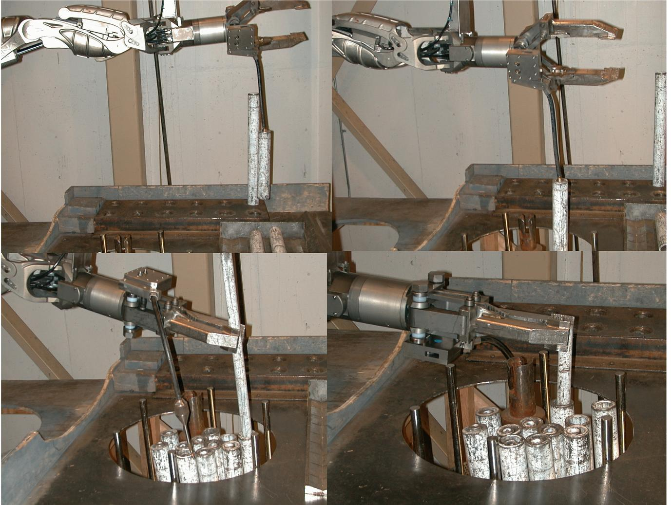
**Figure 12. Loading Fuel into the MCO Fuel Basket.**
