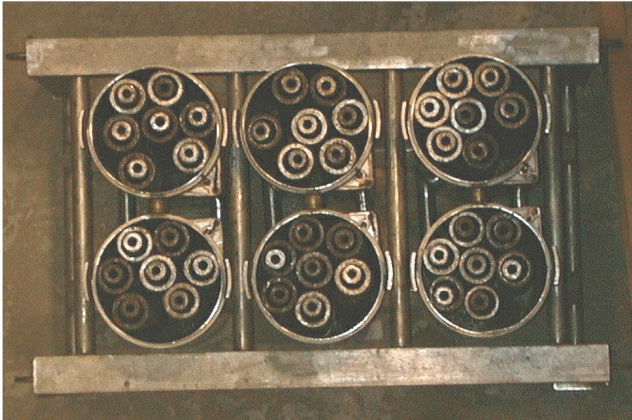
**Figure 2. Fuel Rack Mockup with 3 Full Fuel Canisters.**
