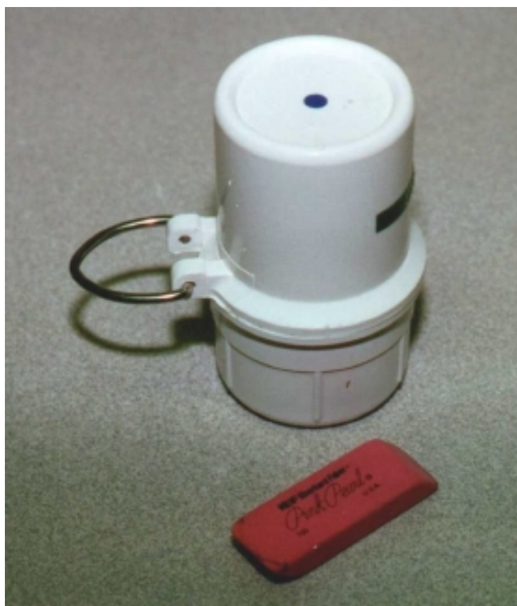
Figure A.5. Temperature Logger Inside of Closed Canister
