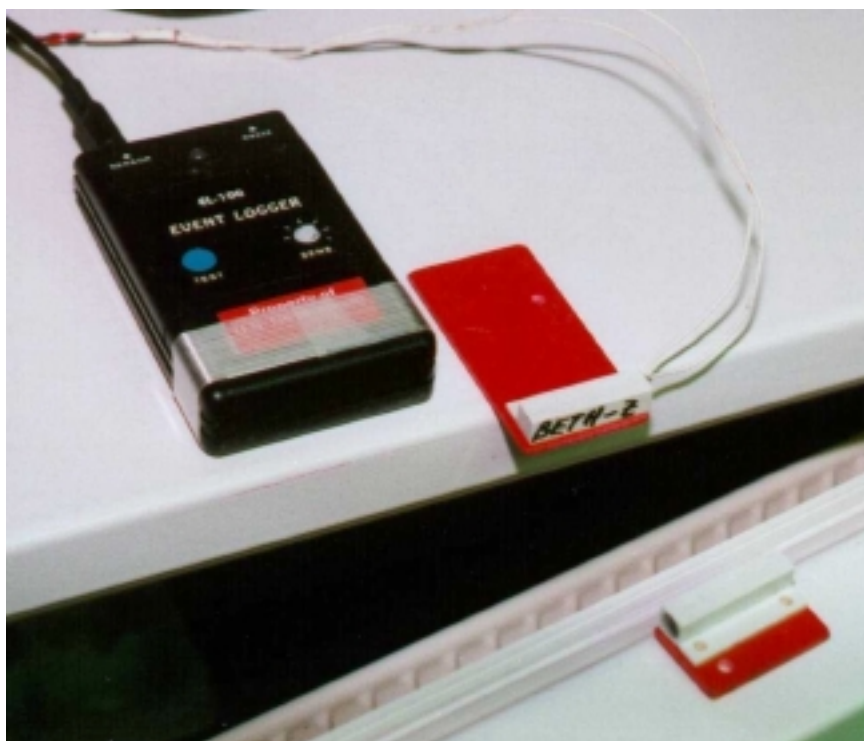
Figure A.3. Event Logger, Magnet, and Reed Switch Mounted on Refrigerator – Refrigerator Door Open
