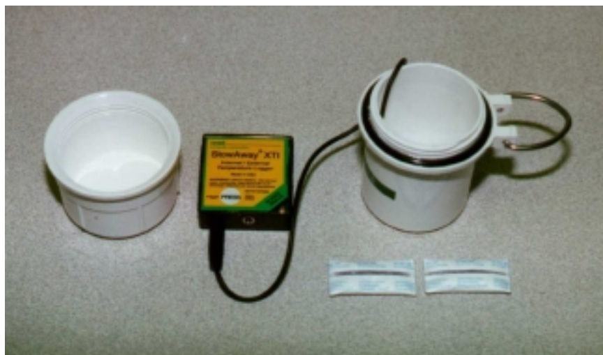
Figure A.4. Temperature Logger, Moisture-Proof Canister, and Desiccant Bags
