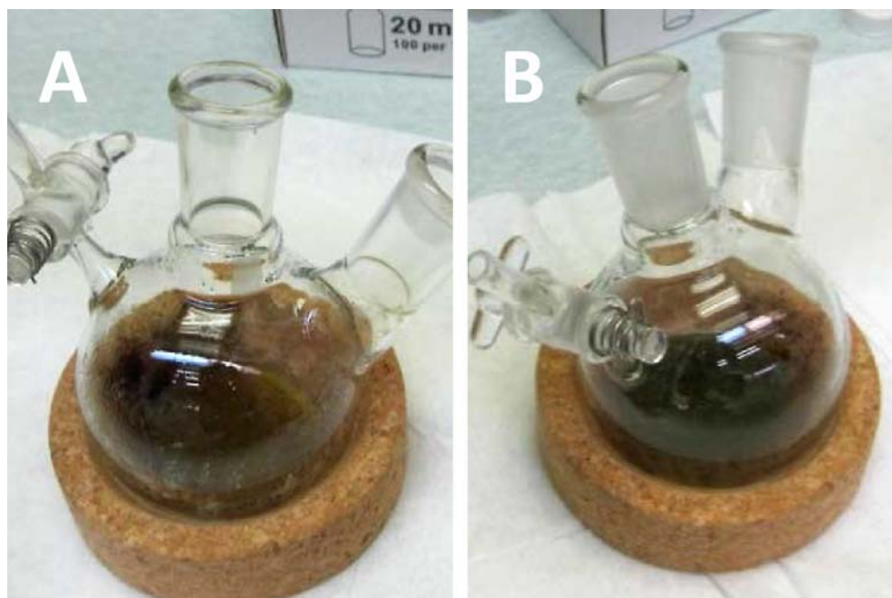
Figure 2.2. (A) Yellow-brown Solution Formed After Dissolving (\text{Bu}_4\text{N})[\text{TcOCl}_4] in Diglyme in Step 2 of Synthesis 9; (B) Dark Brown Solution Resulting from Addition of \text{BH}_3\text{-THF} Solution to (\text{Bu}_4\text{N})[\text{TcOCl}_4] in Diglyme
