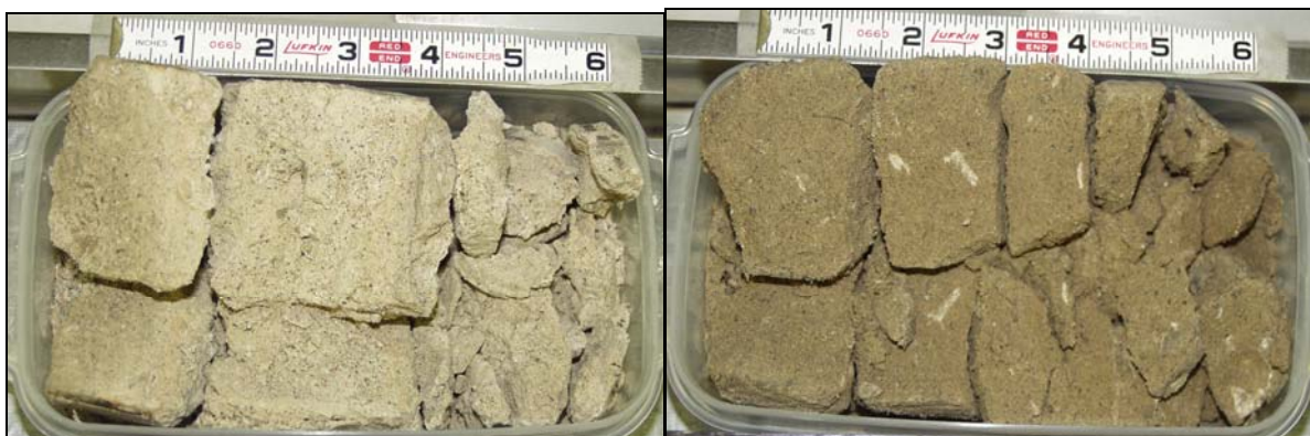
Figure 2.23. Lower Cold Creek Subunit within C4105. Left photo: Core sample S03044-15A from a depth of 102.85 to 103.52 ft bgs. Described as slightly moist, very poorly sorted, moderately cemented, very strongly calcareous, massive, very pale brown, matrix-supported, slightly gravelly sandy mud (gsM). The subtle, diffuse color change at the left end of the core represents a physico-chemical transition between soil horizons. Right photo: Core sample S03044-13A from a depth of 100.00 to 100.68 ft bgs. Described as slightly moist, moderately sorted, moderately to strongly calcareous, weakly to moderately cemented, massive, olive-brown, silty fine-medium sand (mS). Irregular, white fragments are pedogenic, calcium carbonate ( \text{CaCO}_3 ) concretions. The top of the cores are to the right.
