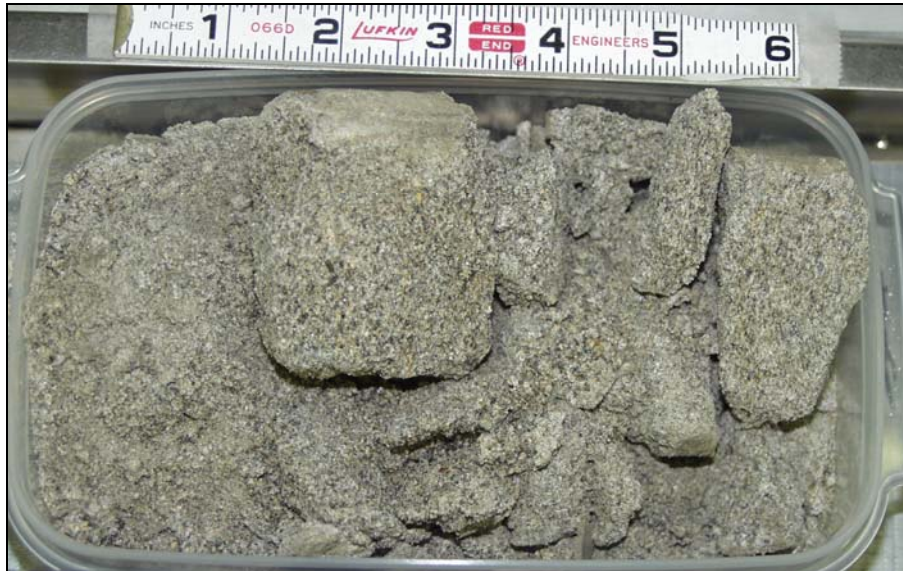
Figure 2.21. Hanford Formation H2 Unit in C4105. Core sample S03044-8A from a depth of 80.88 to 81.58 ft bgs. Described as a slightly moist, loose, moderately sorted, laminated, moderately calcareous, fine to medium, “salt and pepper”-like, grayish-brown sand (S). About 20-30% of the sand grains are dark basalt rock fragments. Light colored grains are mostly quartz and feldspar. The top of the core is to the right.
