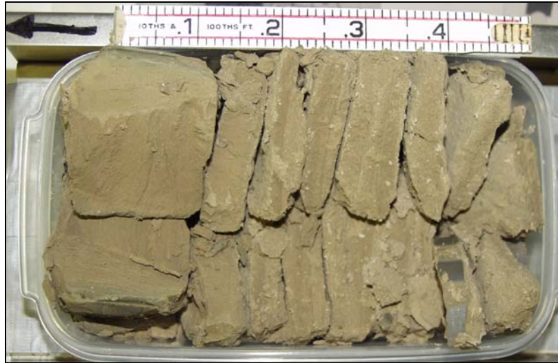
Figure 2.15. Upper Cold Creek Subunit (CCU w ) in C4104. Core sample S03072-11A from 87.0 to 87.7 ft bgs. Described as moist, well laminated, compacted, well-sorted, olive-brown, silt (M) to fine sandy silt (sM), and strongly calcareous. The high concentration of calcium carbonate appears to be the result of erosion and fluvial reworking of the underlying CCU 1 caliche layers, and not from in situ soil development. Top of core is to the right.
