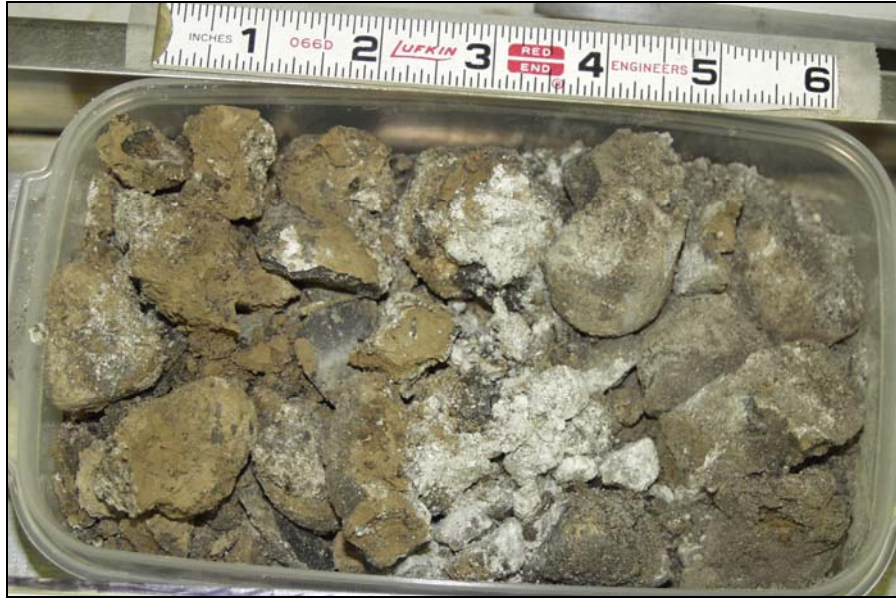
Figure 2.25. Ringold Formation, Member of Wooded Island ( R_{wi} ) in C4105. Core sample S03044-20A from a depth of 123.57 to 124.24 ft bgs. Upper part consists of pulverized, loose, very poorly sorted, non-calcareous, clast-supported, gray, sandy gravel. Lower part is a cohesive, poorly sorted, moderately calcareous, matrix-supported, yellowish-brown, silty gravel. In both parts, gravel clasts are pulverized and consist of 40-60% basalt. The light colored material through the middle is the remains of a pulverized granitic or quartzite clast, crushed during drilling. The top of the core is to the right.
