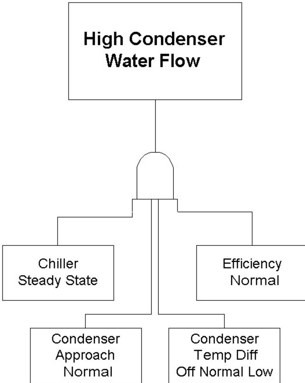
Figure 4: Logic block diagram for High Condenser Water Flow
