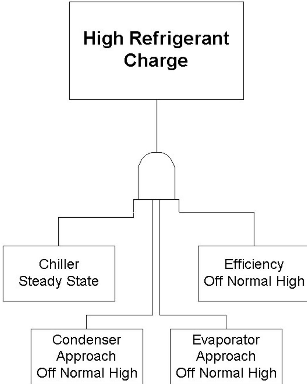
Figure 6: Logic Diagram for High Refrigerant Charge Diagnostic
