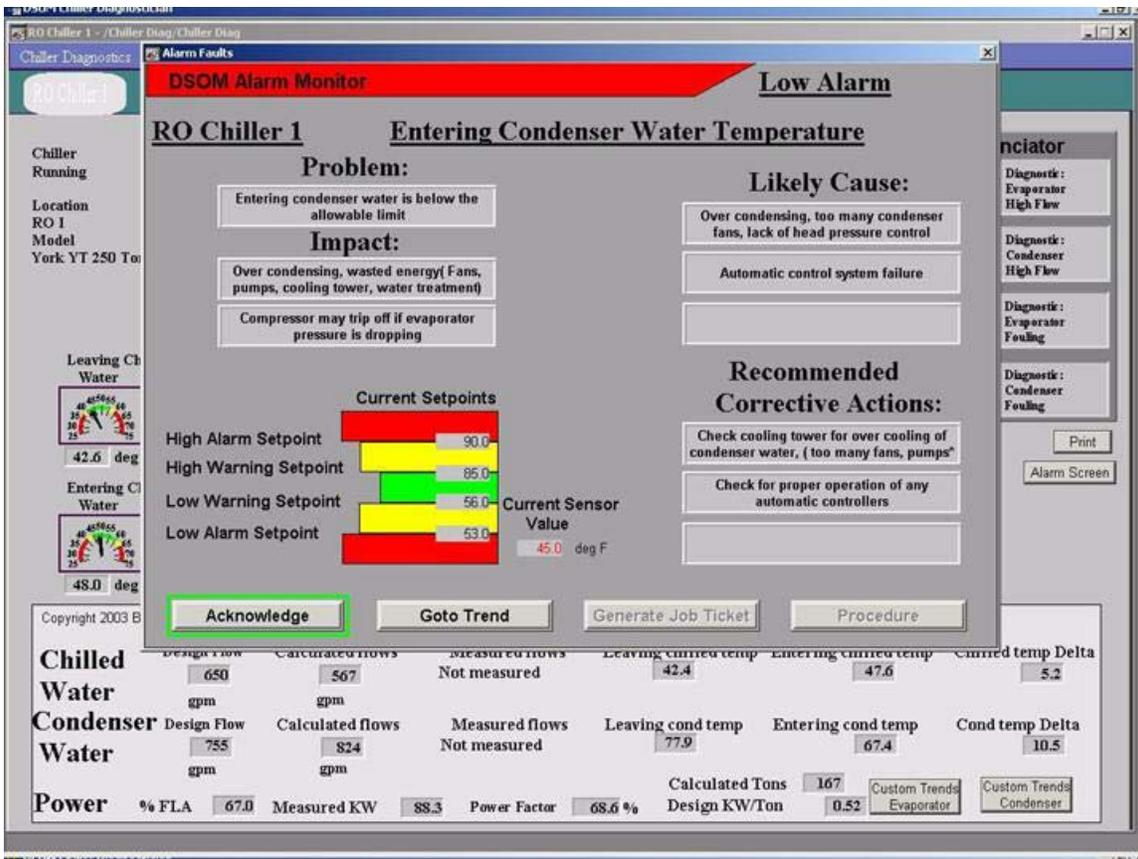
Figure 2: Chiller Diagnostician Alarm Display
