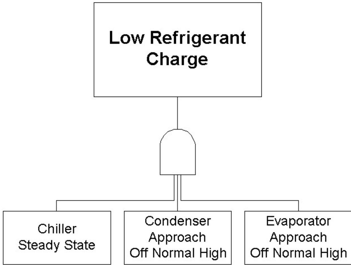
Figure 5: Logic Diagram for Low Refrigerant Charge Diagnostic
