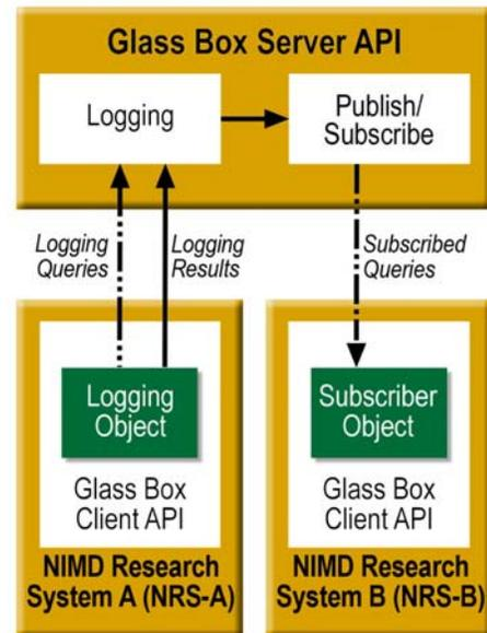
**Figure 4: Using the Glass Box API to log and subscribe**
