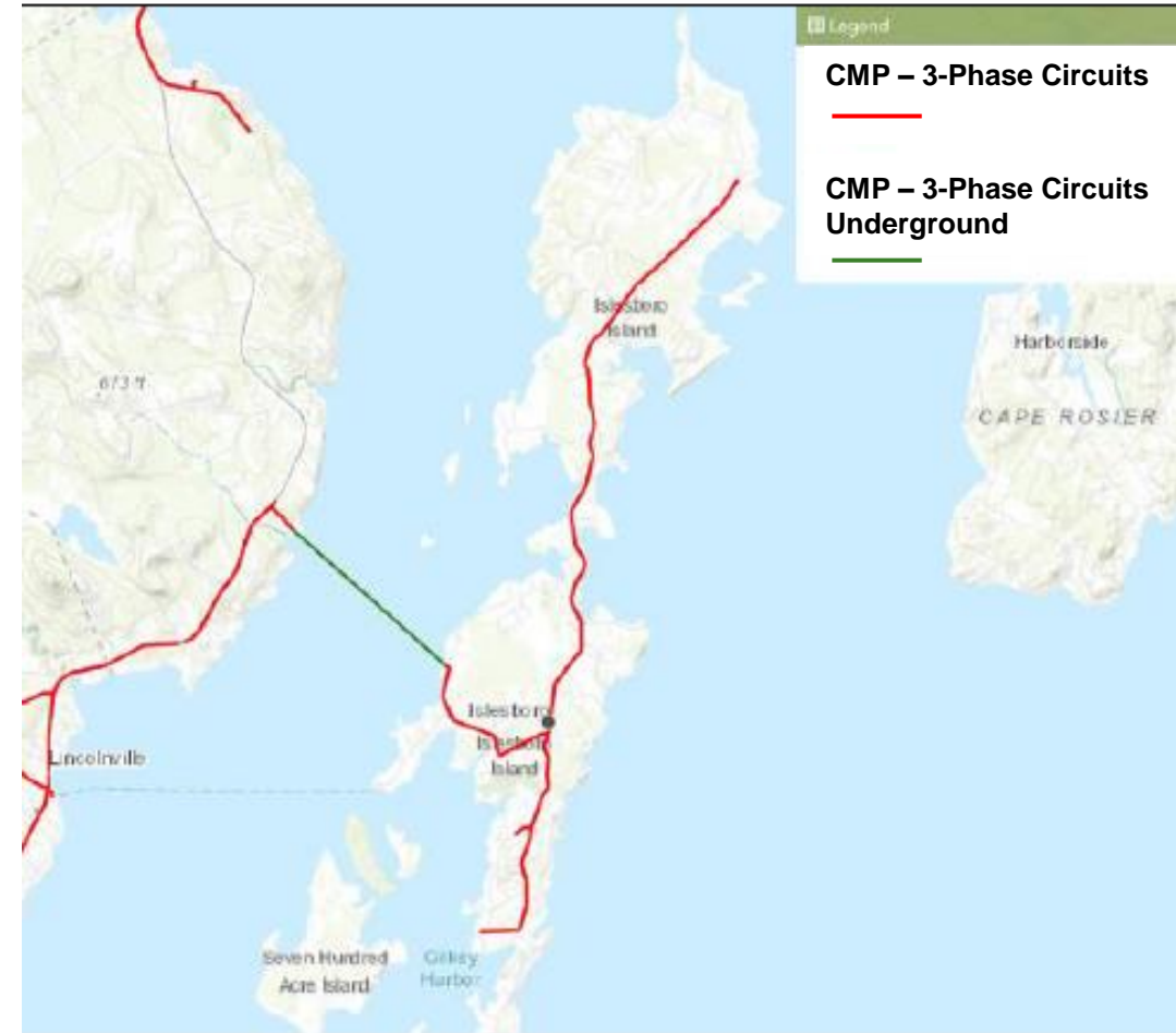
Three-phase circuits by CMP on Islesboro
