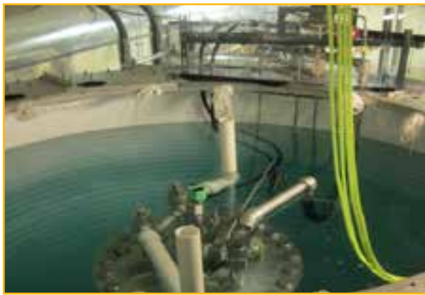
COUPP60 Bubble Chamber—now taking data at SNOLAB
