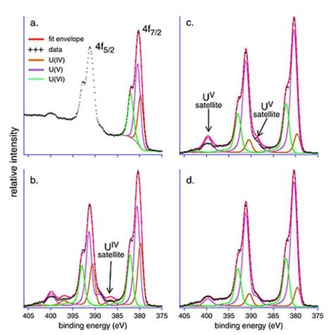
The team elucidated a systematic approach for identifying uranium's state and hence mobility using x-ray photoelectron spectra, such as these shown for a sodium, uranium, oxygen compound on silica.
