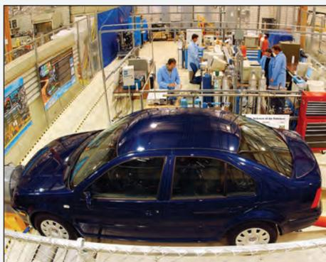
At PNNL's exhaust emissions laboratory, researchers can use a suite of instruments to develop and evaluate vehicle exhaust after-treatment systems. As seen here, a diesel car can be on a chassis dynamometer—a treadmill for vehicles that provides realistic road operating conditions for testing new technologies.
