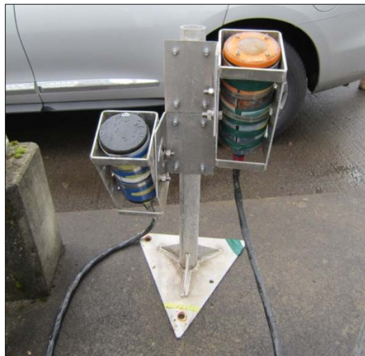
Figure 6. Example of single-beam transducer mount that could be used at spill bays.
