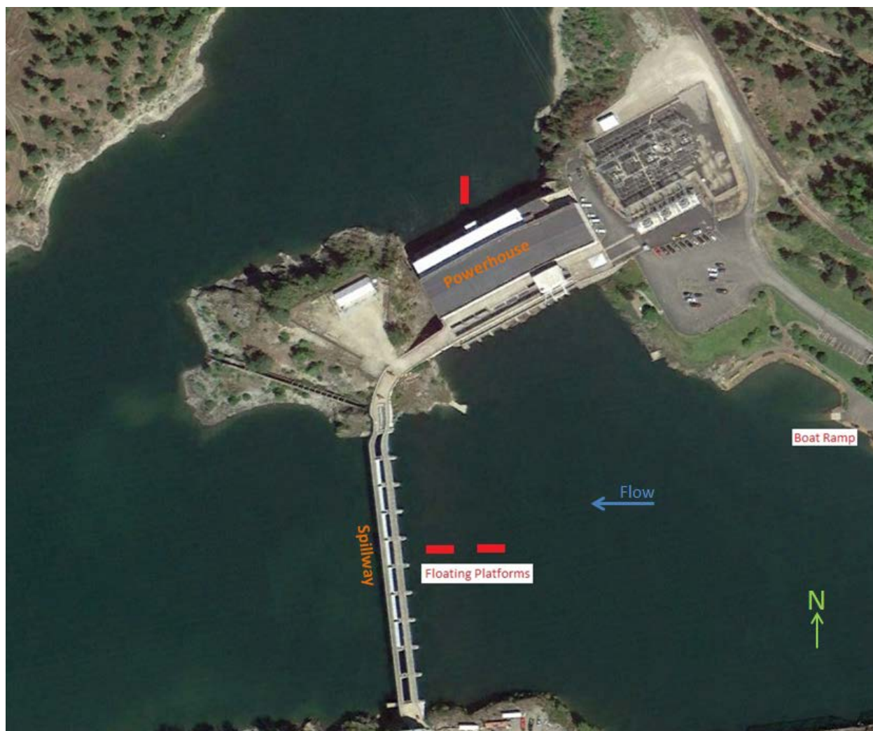
Figure 4. General configuration of the floating platform locations that would be attached to a fyke net sampling a spill bay of Albeni Falls Dam (two horizontal red dashes) or attached to the cod-end of a net sampling a turbine draft tube (vertical red dash).
