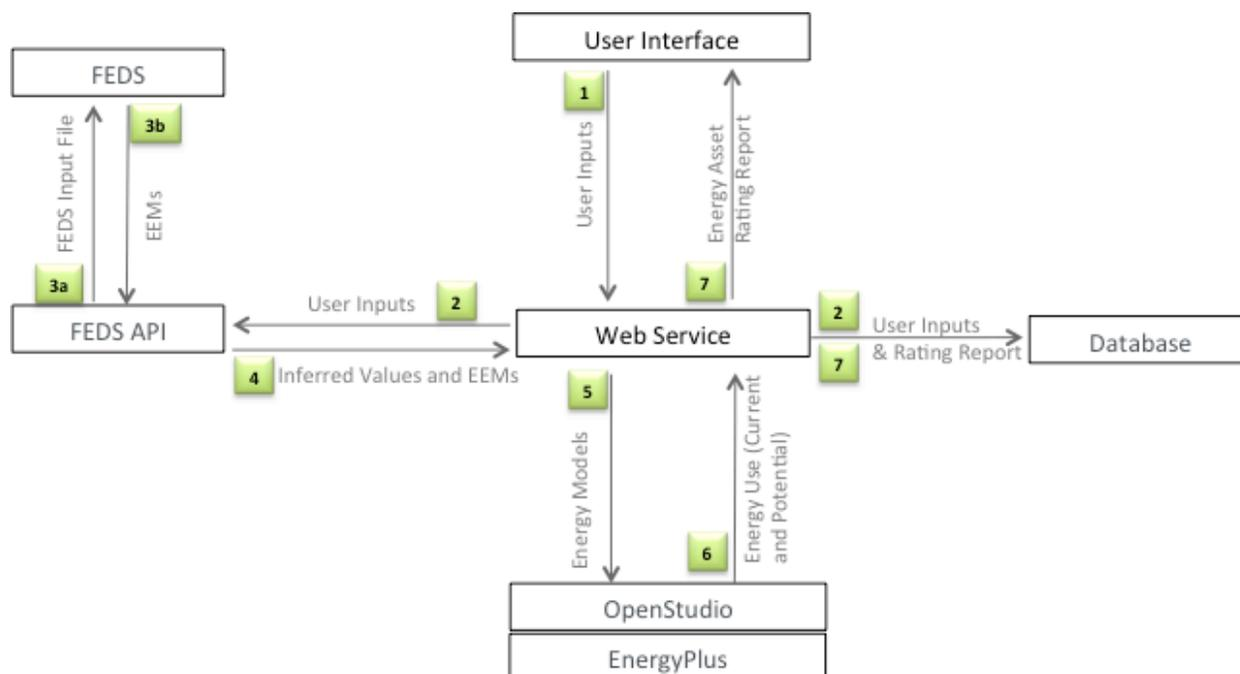
Figure 4.4. Energy asset scoring tool architecture.
