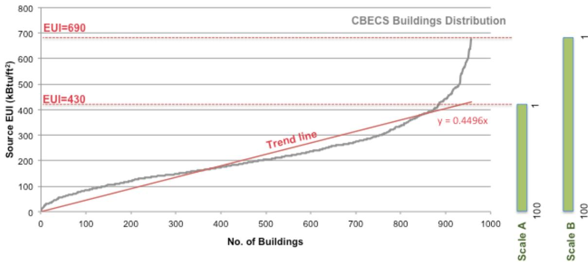
**Figure 3.8.** Office building scale development based on CBECS 2003 data.
