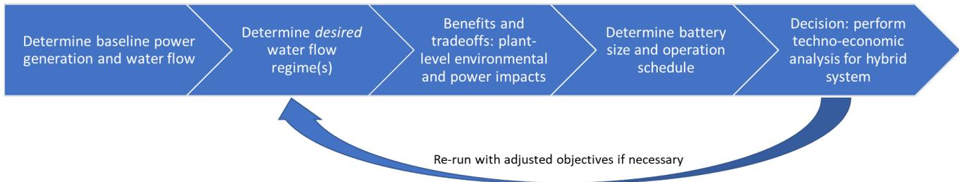
Figure 2. Energy storage sizing methodology.
