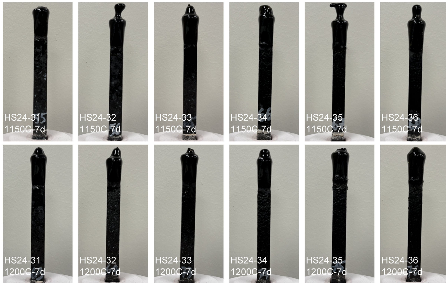
Figure A.6. K-3 coupons HS24-31 through HS24-36 after the refractory corrosion test.
