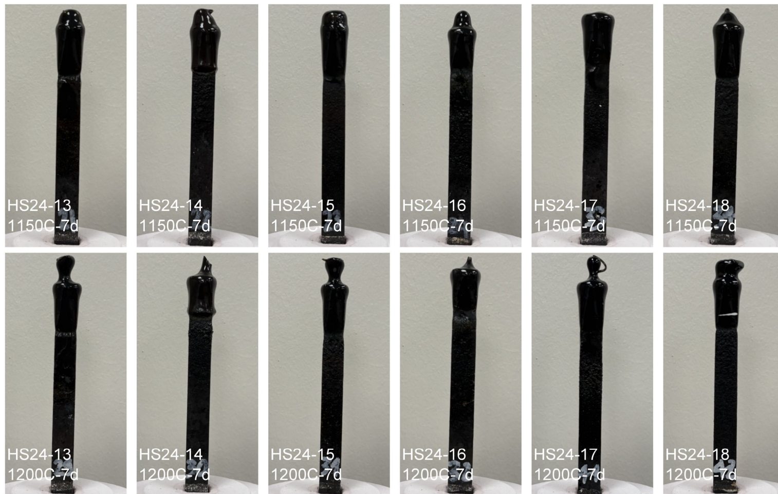
Figure A.3. K-3 coupons HS24-13 through HS24-18 after the refractory corrosion test.
