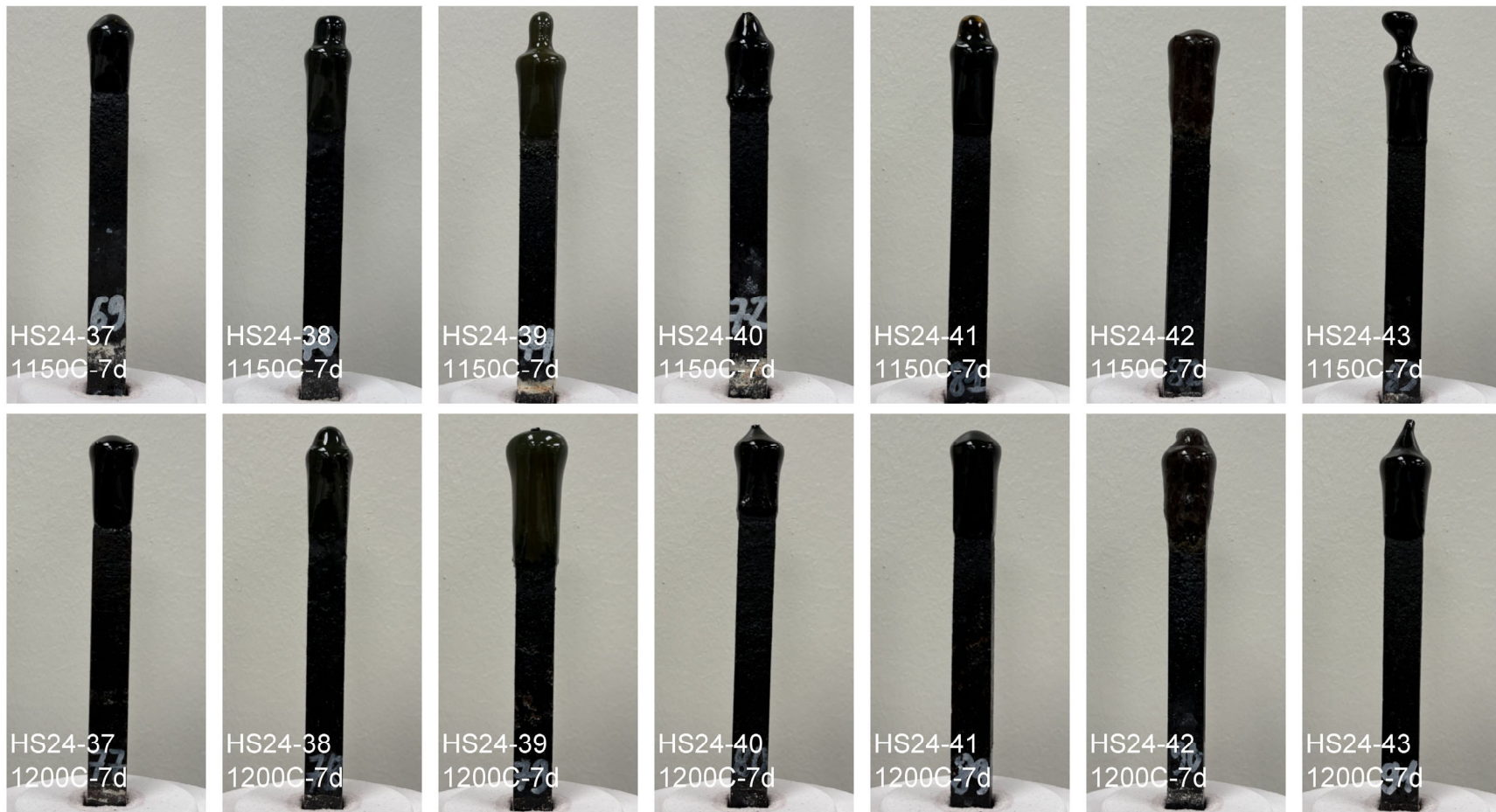
Figure A.7. K-3 coupons HS24-37 through HS24-43 after the refractory corrosion test.
