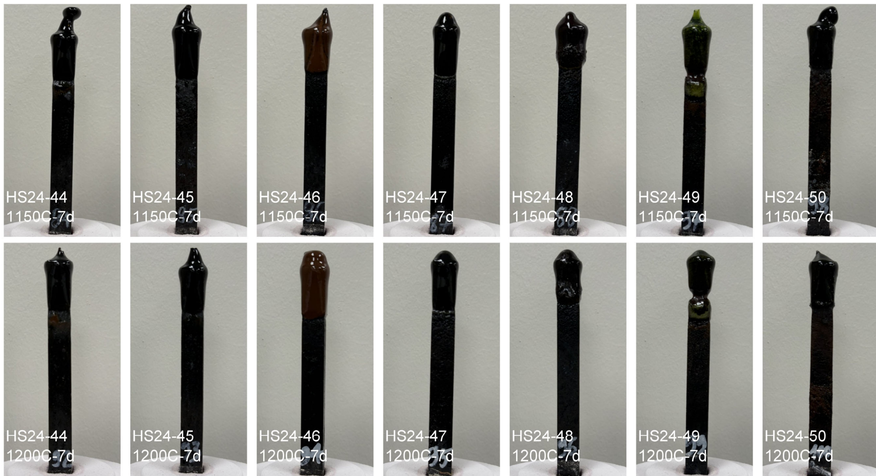
Figure A.8. K-3 coupons HS24-44 through HS24-50 after the refractory corrosion test.
