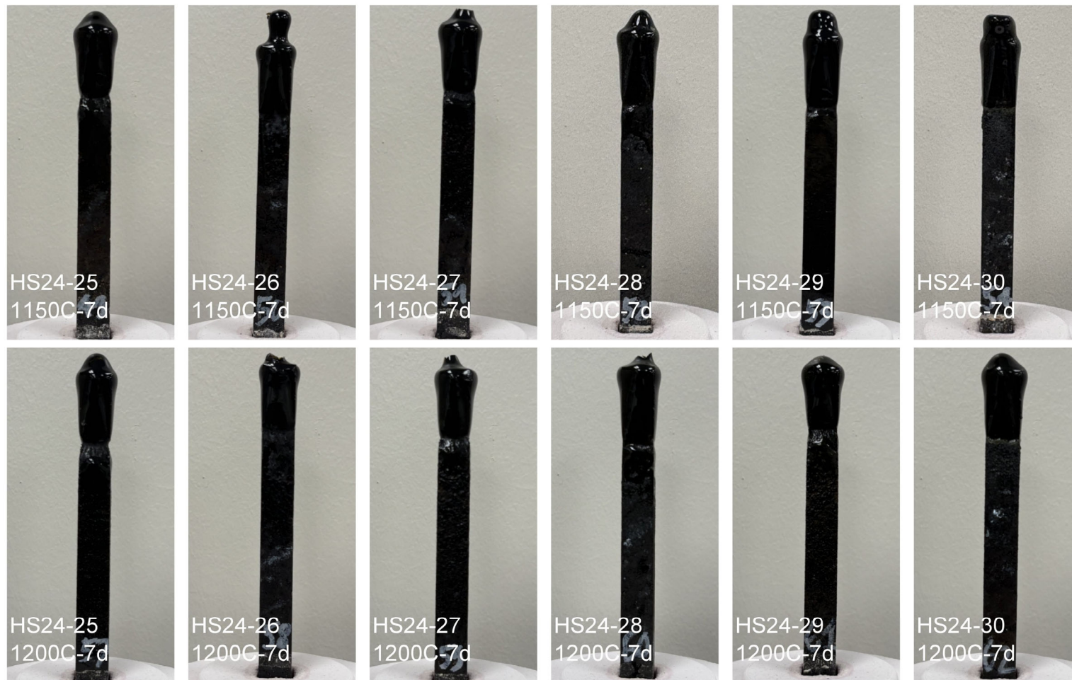
Figure A.5. K-3 coupons HS24-25 through HS24-30 after the refractory corrosion test.
