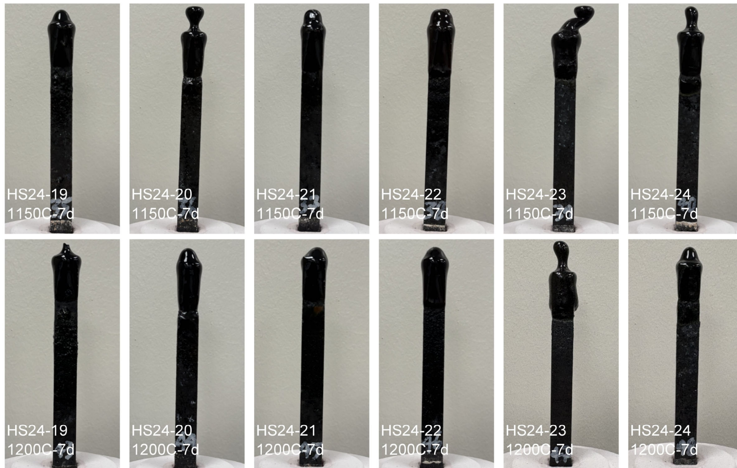
Figure A.4. K-3 coupons HS24-19 through HS24-24 after the refractory corrosion test.
