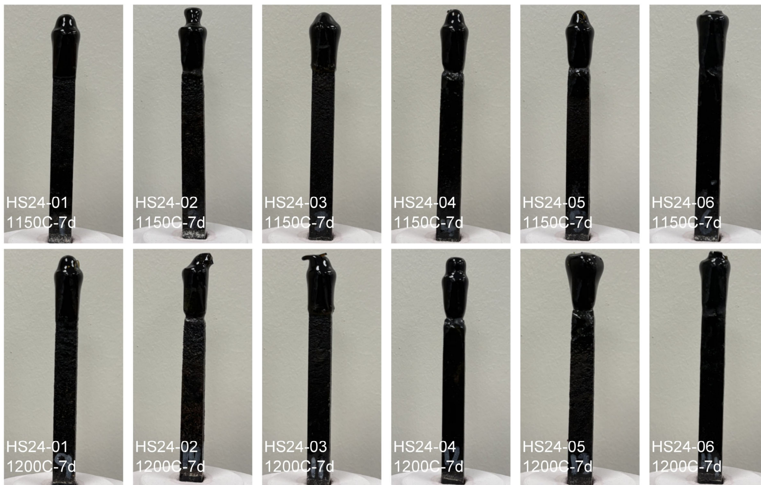
Figure A.1. K-3 coupons HS24-01 through HS24-06 after the refractory corrosion test.
