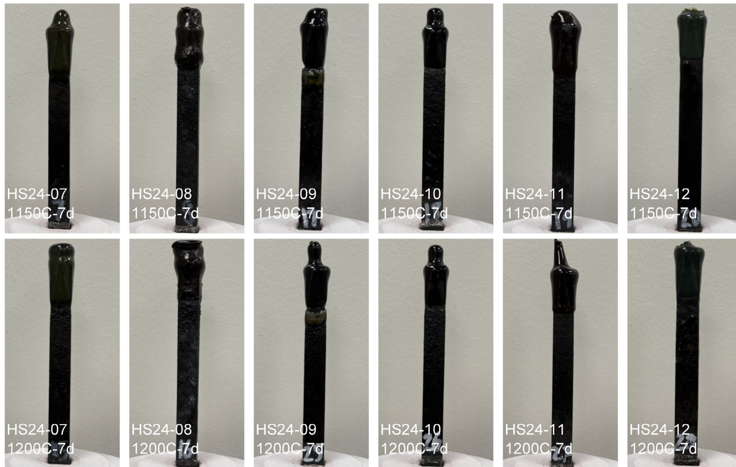
Figure A.2. K-3 coupons HS24-07 through HS24-12 after the refractory corrosion test.
