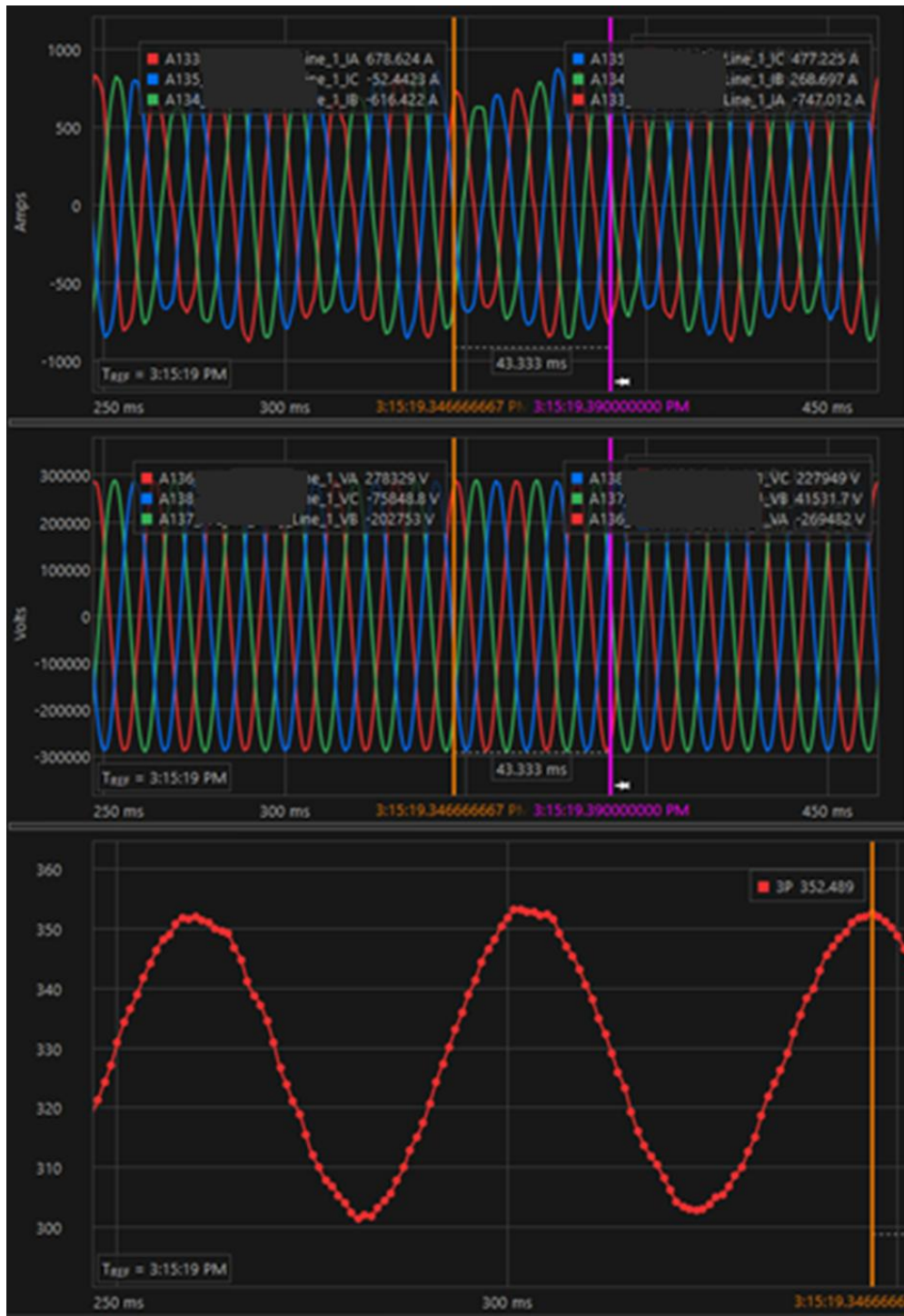
Figure 2. Large load oscillation event at ERCOT observed from 20 samples/cycle DFR measurements. The red trace in the bottom plot is three-phase power and reveals the 50 MW oscillation. Source: ERCOT (Gravois 2025).
