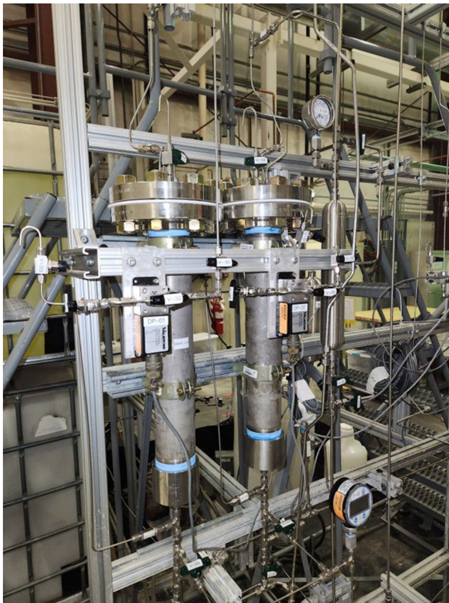
Figure 3.4. Image of the as-assembled 200W-scaled DEFs installed in the system (LS2 configuration). DEF-01 is on the left and DEF-02 is on the right in the image.
