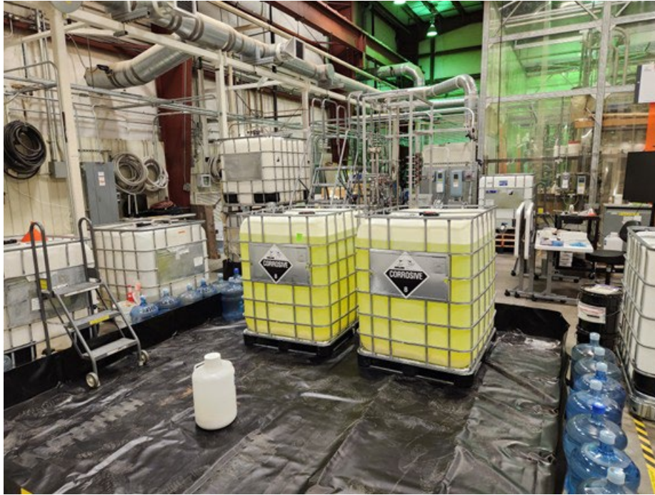
Figure 3.7. Experimental system workspace in PDLE facing north. Feed simulant IBC totes shipped from the vendor are in the foreground, with the experimental system (in the LS1 configuration) immediately behind. The IBC totes on the left edge of the image were used for capturing process and effluent solutions as each experimental run progressed.
