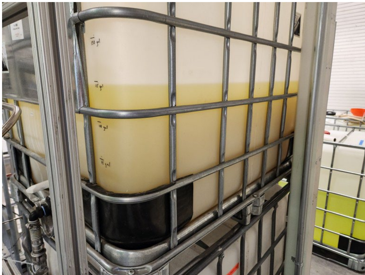
Figure 4.1. Close-up of S2 simulant in TK-01 during experimental W-02. Contrast the color and opaqueness of the solution in the foreground to the material in the IBC tote in the background, which is filtered S2 liquid.
