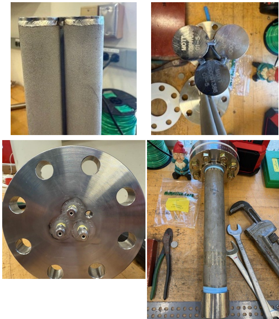
Figure 3.3. Images detailing the 200W-scaled DEF fabrication. Clockwise from the top left: Side view of the filter elements with welded spacers, top view of the filter elements welded to the flange, full DEF assembly, and top view of the filtrate discharge ports and vent port.
