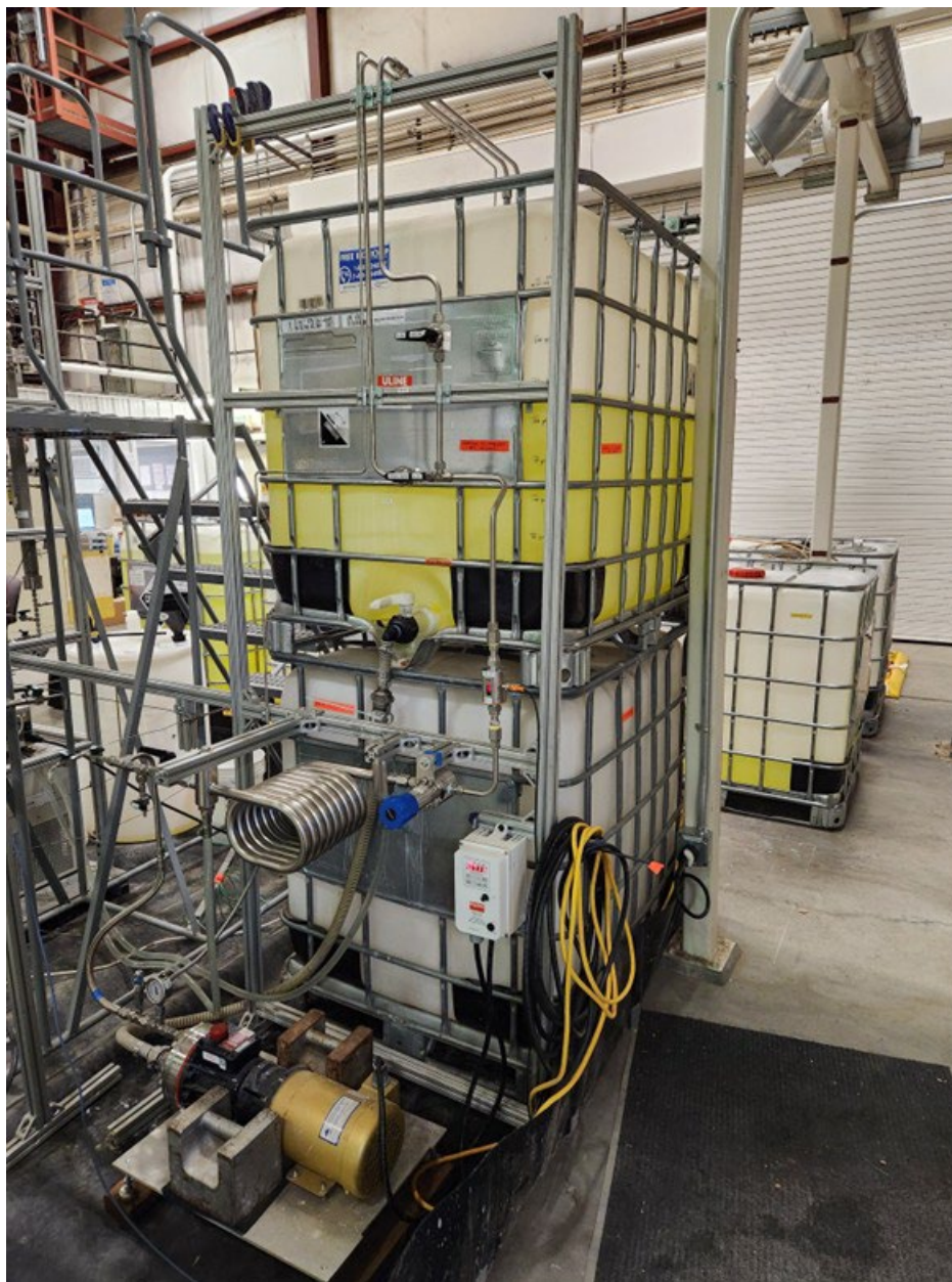
Figure 3.10. Feed vessel (TK-01) and recirculation loop of the experimental system facing south. On the ground in front of the stacked totes is PMP-01, with TK-01 being the upper tote (partially filled with simulant). The elements of this part of the system were unchanged across the LS1 and LS2 configurations.
