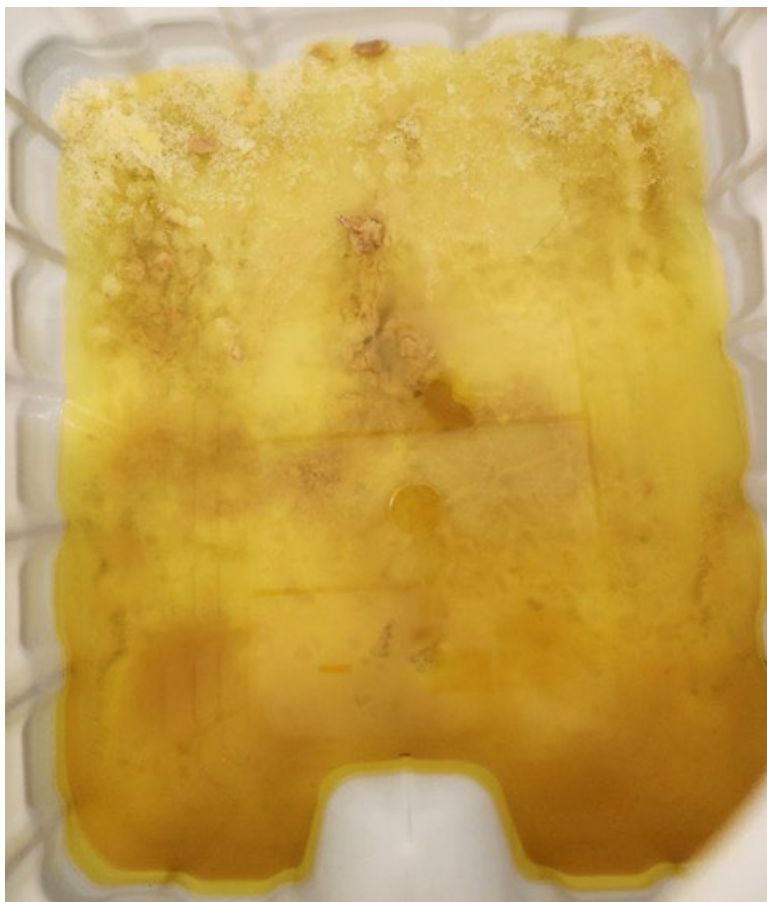
Figure 6.6. S1 IBC tote with residual solids.
