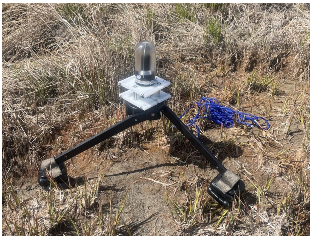
Figure 2. Hydrophone lander prior to deployment with weights on the foot of each tripod leg. The icListen HF SC2 hydrophone, equipped with a flow shield, is shown.
