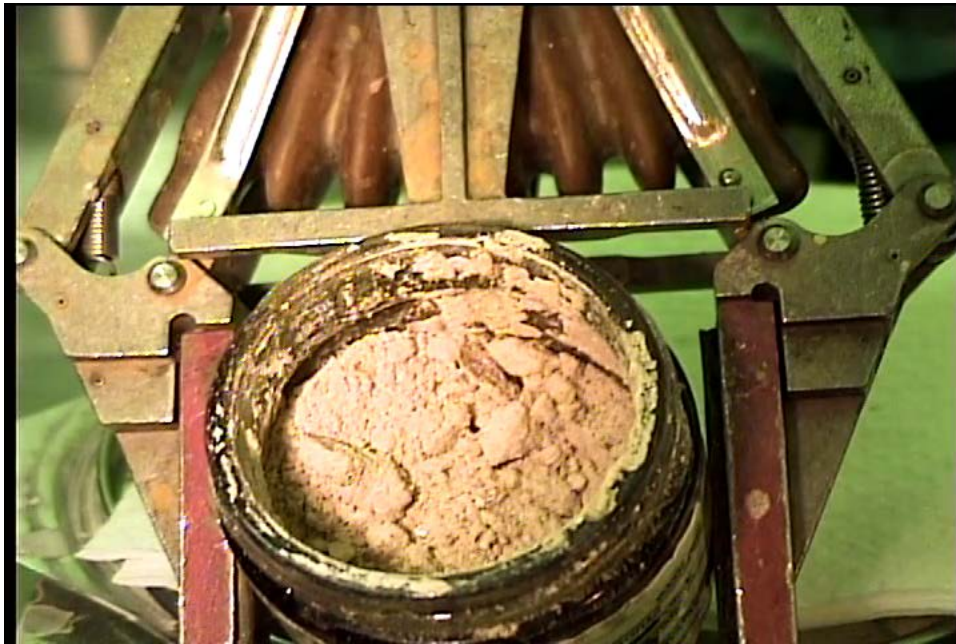
Figure 4. Image of solids within Jar 21415 (AN-101 Segment 18 LH). The solids appear dry powder with intermediate-sized aggregates.
