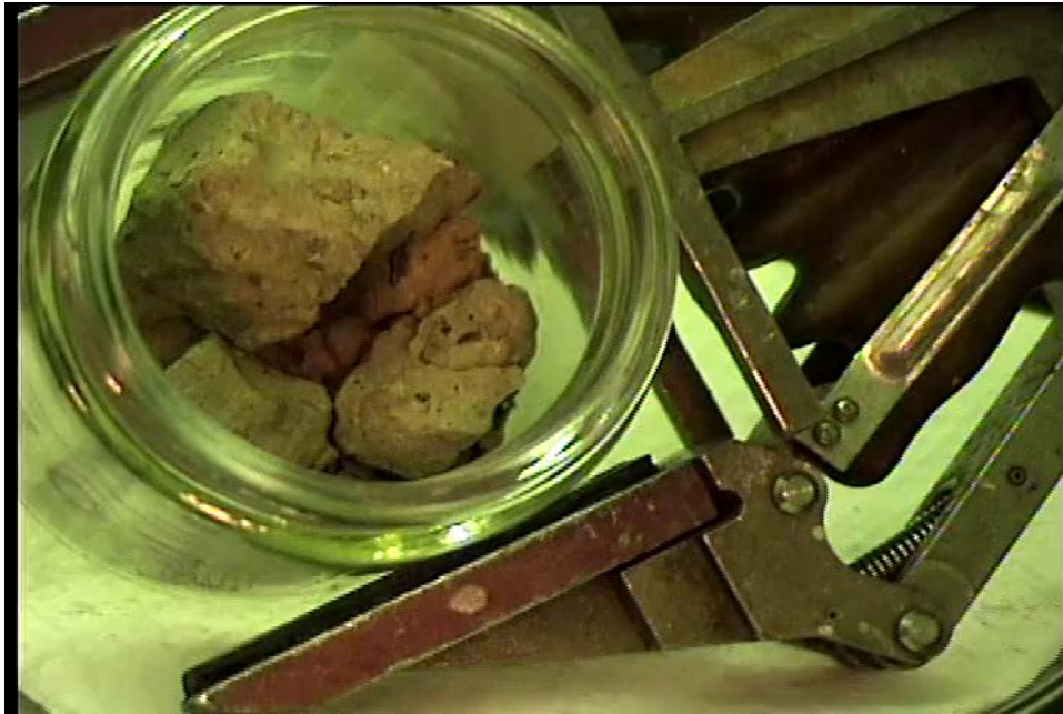
Figure 6. Image of solids within Jar 20507 (AW-105 Segment 8R2). The solids appear as large aggregates.
