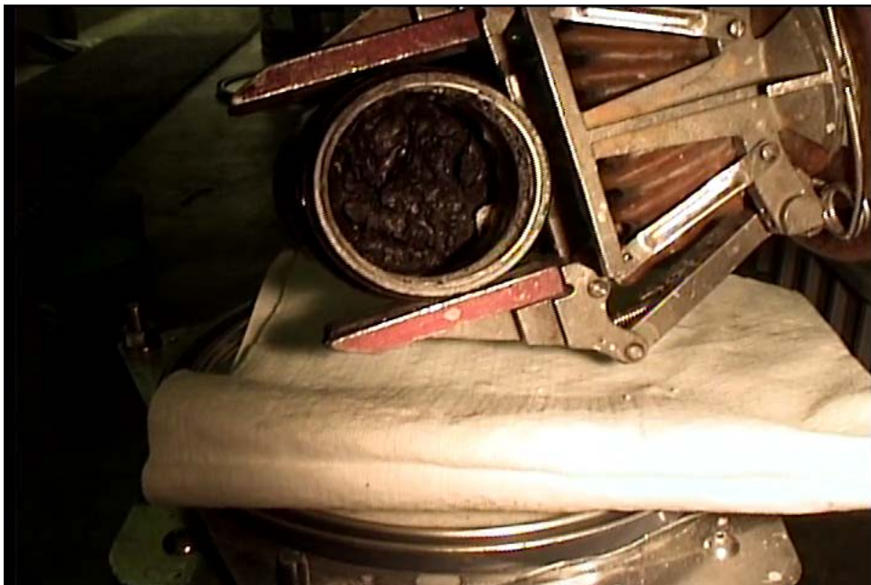
Figure 9. Image of solids within Jar 20326 (AW-105 Segment 8 LH). The solids exhibited a dense paste-like consistency with limited inherent moisture.
