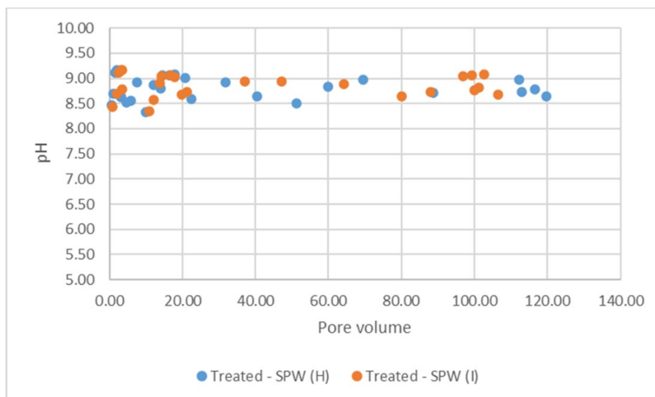
Figure F.30. pH during loading and leaching with PZsd sediment and CoCOIs with Sn(II)-PO 4 treatment.
