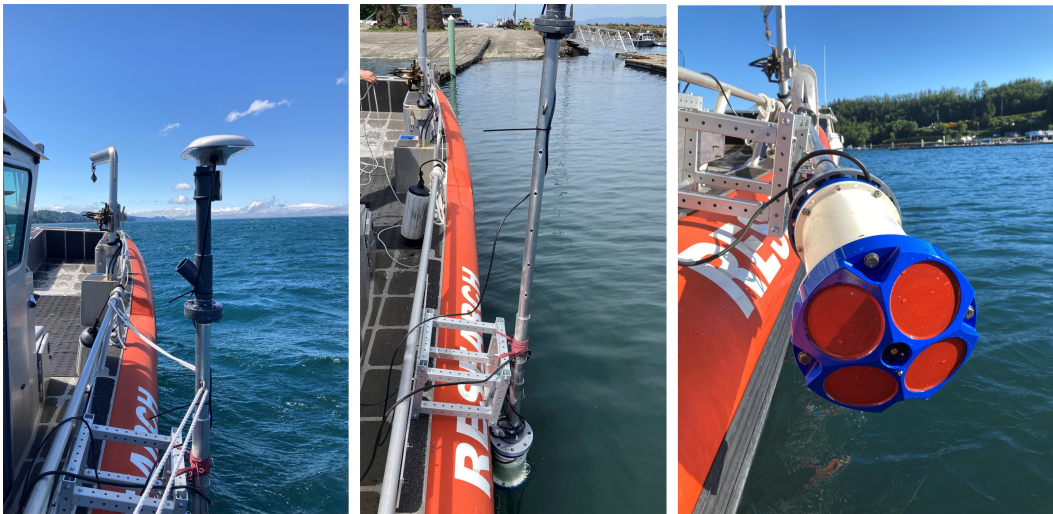
Figure 8. ADCP and GPS mounted on the survey vessel, R/V Desdemona. Left: active surveying, Center: pole-mount in raised position at dock, Right: pole-mount rotated 90 degrees in transit position
