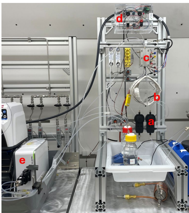
Figure 3: Photograph of the assembled electrochemical reactor platform showing: (a) liquid pumps, (b) liquid pre-heating loop, (c) electrochemical flow cell, (d) electronic control panel for liquid pumps, (e) ReactIR equipped with a flow detector, (f) potentiostat (not shown).
