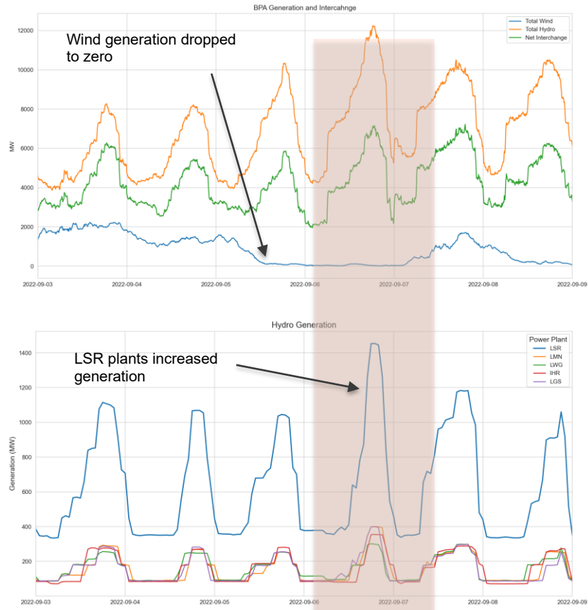
Figure S.5 BPA total generation, net interchange, and LSR plants generation during peak load in California.
