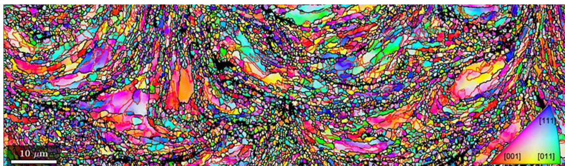
Figure 3. Electron backscatter diffraction of cold sprayed nickel-yttria (Gwalani et al. 2022)
