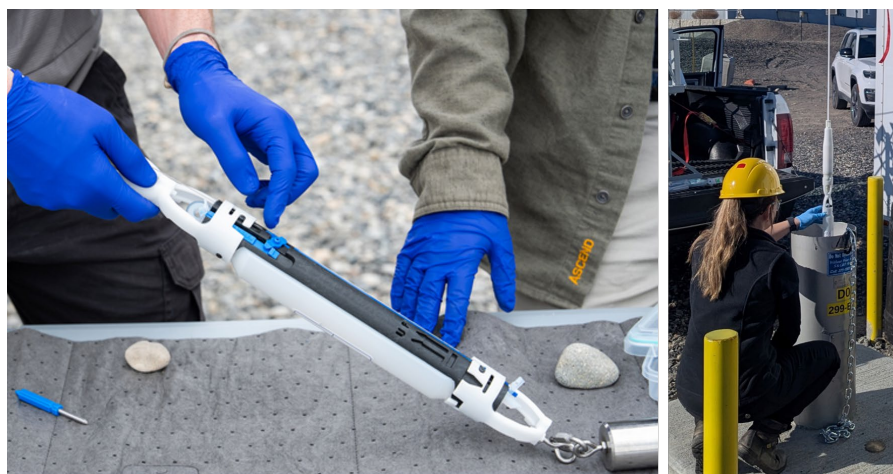
Figure 5. Snap sample construction (left); snap sample deployment (right).
