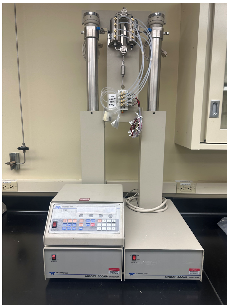
Figure 2. Dual ISCO syringe pumps used for flow control.
