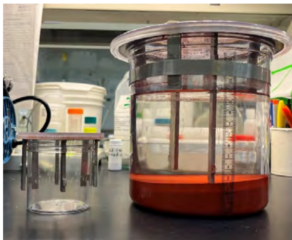
Figure 2.1. Small-scale tank (left) and bench-scale tank containing melter feed preparation vessel simulant (right).
