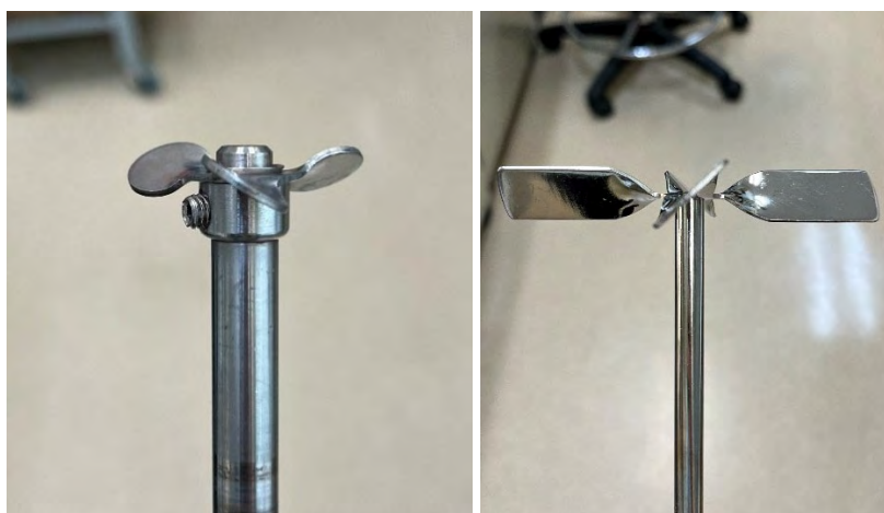
Figure 2.2. Cole-Parmer 316 stainless steel three-blade propeller, 1-1/2 in. diameter x 5/16 in. bore diameter (left), and IKA R 1345 propeller 4-bladed stirrer (right).
