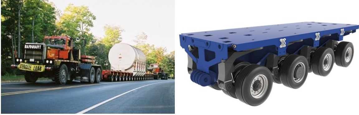
Figure 1-8. Transportation options—Heavy-haul truck (left) and self-propelled modular transporter (right).
