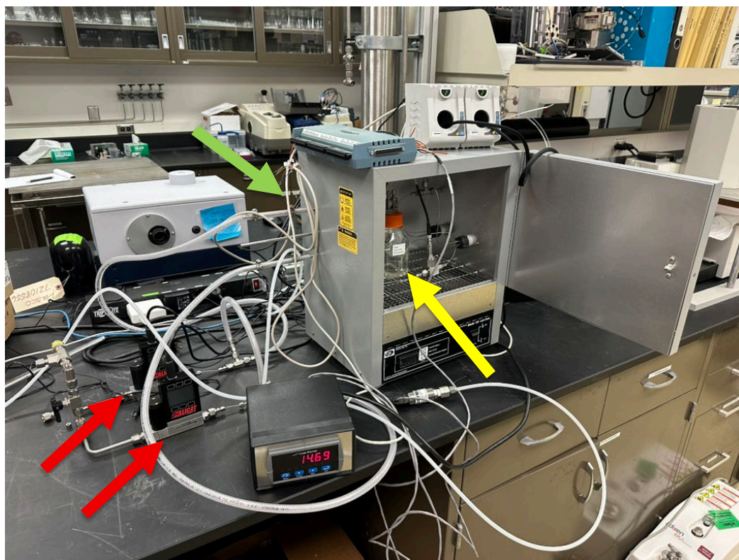
Figure 3. Mass flow-controller system for generating gas streams at specified relative humidity (RH). Red arrows indicate the mass flow controllers, the green arrow indicates the oven, and the yellow arrow indicates the water vessel containing the semipermeable Nafion tube for humidification.
