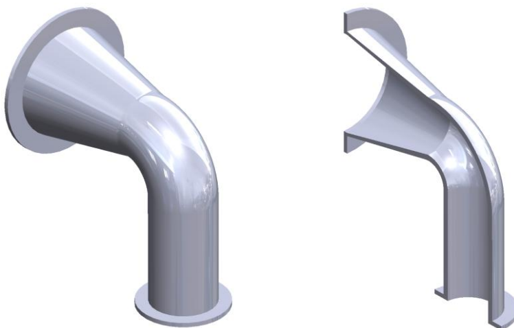
Figure 4. Draft Schematic of Expanded Elbow Pipe
